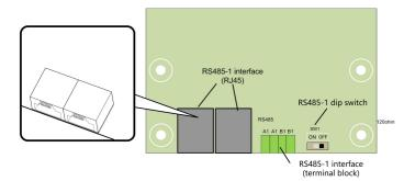
All three interfaces can be connected to a data acquisition device (Data Logger), to achieve data exchange with PC or other monitoring devices.
