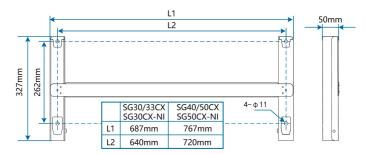
figure 4-1 Dimensions of Mounting-bracket
