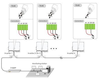
figure 5-5 Multi-inverter Connection
