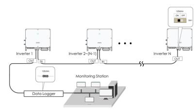
figure 5-6 Configuration of Dip Switch (N≥15)
