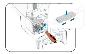
step 4 Pull out the fan module, clean the fans with soft brush or vacuum cleaner, and replace them when necessary.
