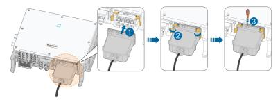
step 8 Gently pull the cable backwards to ensure firm connection, and fasten the swivel nut clockwise.
