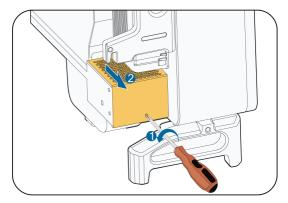
step 3 Press the tab of the latch hook, unplug the cable connection joint outwards, and loosen the screw on the fan holder.
