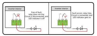
figure 5-7 Normally open contact
