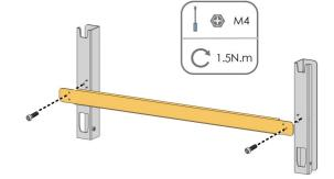
step 2 Level the assembled mounting-bracket by using the level, and mark the positions for drilling holes.
