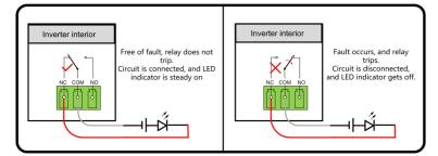
figure 5-8 Normally closed contact
