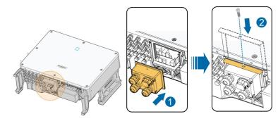
During installation, firmly press the junction box to ensure that the pin can be inserted successfully.
