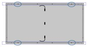
Installation with bolts into 4 outer holes
