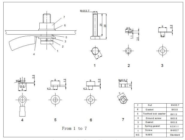
Figure 5.Example of acceptable ground connection
