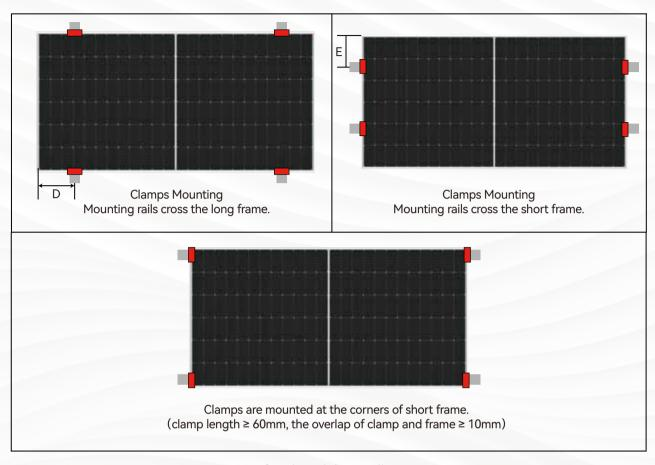
Figure 7 Mono-facial Module Installation Position
