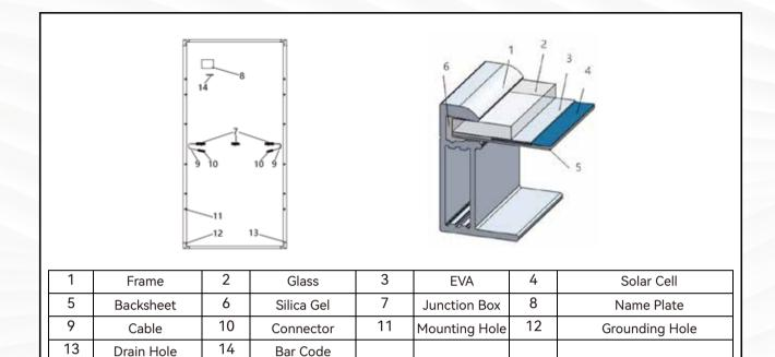
Figure 1 Typical Mechanical Drawing of Mono-facial Modules
