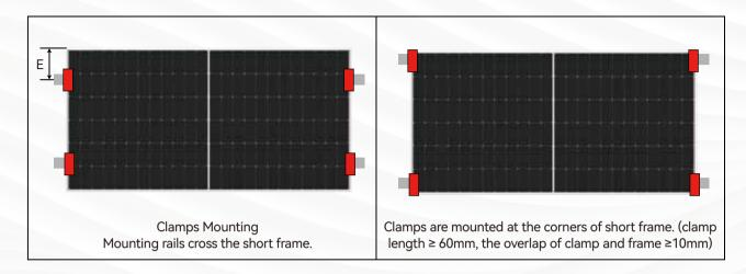
Figure 8 Bifacial Module Installation Position
