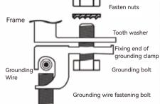
Figure 10 Bolt Grounding Method of PV Module
