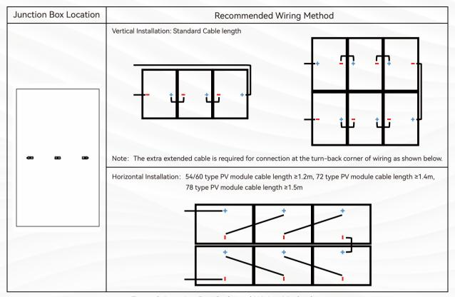
Figure 3 Junction Box Style and Wiring Method
