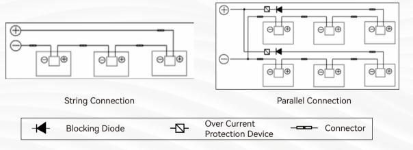
Figure 9: Series Connection and Parallel Connection Circuit Diagram
