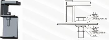
Figure 5 Bolt Installation of Mono-facial Modules
