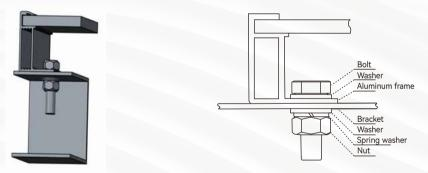
Figure 5 Bolt Installation of Mono-facial Modules
