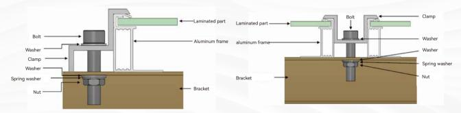
Figure 6 Clamp Installation of Mono-facial Modules
