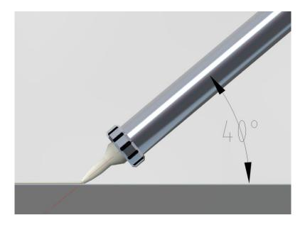
Adhesive size and standard dosage: at least 10\*5mm; 5 strips/1 module (adhesive along the width of the PV module); 3 strips/1 module (adhesive along the length of the PV module)
