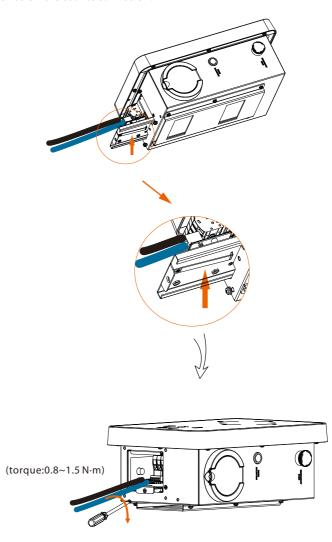
STEP 11: Push the rear cover to appropriate position of the cables and screw the self tapping screws with the cross screwdriver. Then tighten the waterproof fastening head.
