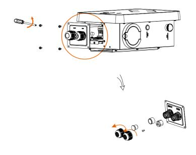
STEP 5: Unscrew the countersunk screw of the base plate of communication board with the cross screwdriver. Then pull the base plate of communication board out.
