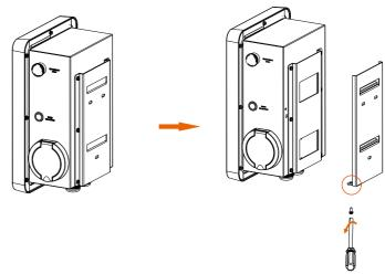
STEP 2: Fix the back bracket and the cable hook (only for Plug Type) to the wall.
