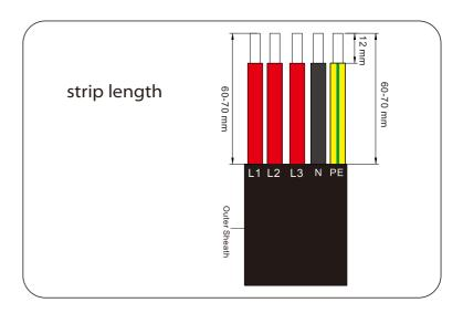
STEP 8: Insert the input cable through the waterproof connector in sequence as shown below.
