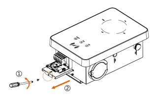
STEP 6: Insert the prepared communication cable through the waterproof connector in sequence as shown below (If the cable is self-made, also insert the wires into the RJ45 terminals and then use crimping pliers to press them tightly).
