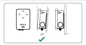
Figure 6-1 Correct installtion
