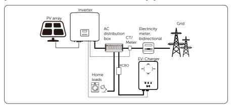
Figure 6-4 Home scene and communication with inverter
