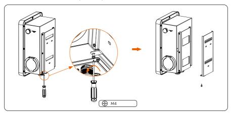
Figure 6-6 Remove the back bracket away
