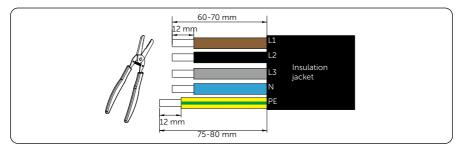
Figure 6-13 Strip the AC input cable
