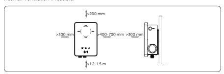
Figure 4-2 Clearance requirement
