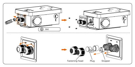
Figure 6-11 Take down and dissassemble the rear cover
