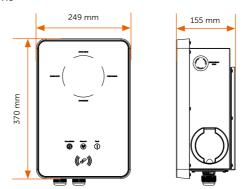
Figure 2-5 Dimensions of Socket Type
