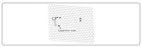
Figure 6-9 Insert the expansion tubes
