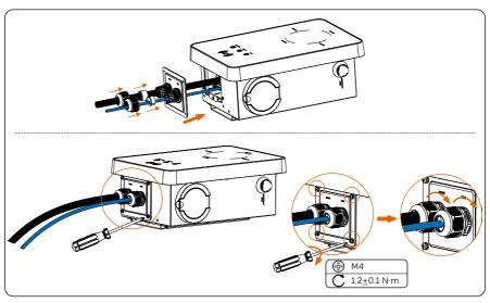
Figure 6-28 Secure the rear cover
