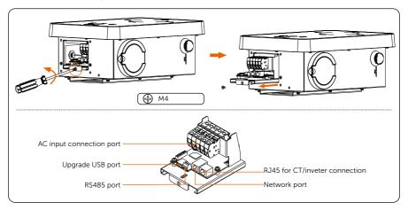
Figure 6-12 Pull the base plate of communication board out
