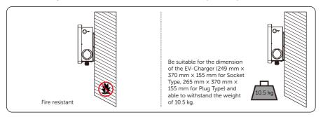
Figure 4-1 Installation carrier requirement
