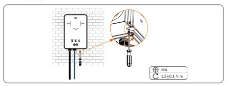
Figure 6-29 Hang and steady the EV-Charger
