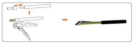
Figure 6-14 Crimp the wires
