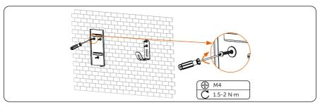
Figure 6-10 Secure the bracket and the cable hook
