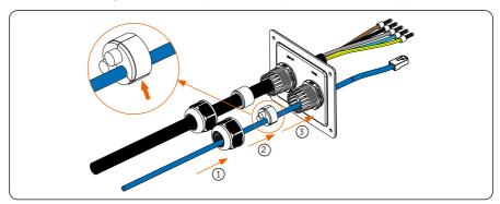
Figure 6-18 Thread the communication cable
