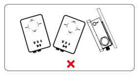
Figure 6-2 Incorrect installation
