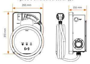
Figure 2-6 Dimensions of Plug Type
