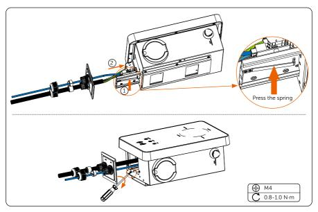
Figure 6-27 Screw the the base plate of communication board
