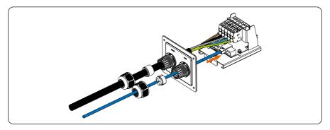
Figure 6-25 Connect the communication cable to Network port
