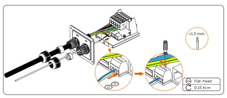
Figure 6-24 Connect the communication cable to RS485 port
