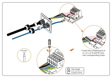
Figure 6-19 Connect the AC input cable
