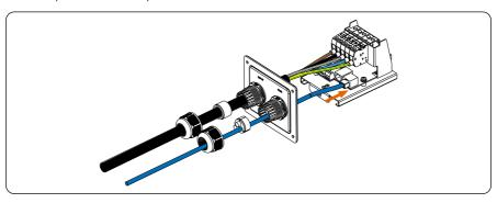
Figure 6-21 Connect the communication cable to RJ45 port
