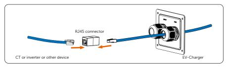
Figure 6-26 Using RJ45 connector
