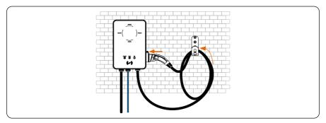
Figure 6-30 Connect the charging connector and hang the cable
