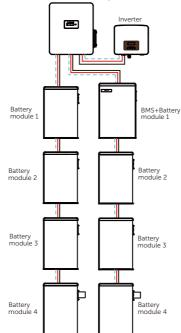
② Connect with T-BAT-SYS-HV-3.0 Connect with a MC0600 (BMS)
