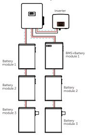
Connect with a T-BAT H 5.8 (BMS) and 3 HV11550 battery modules:
