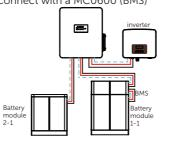
Connect with a MC0600 (BMS) and 4 HV10230 battery modules:
