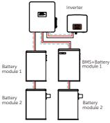
Connect with a T-BAT H 5.8 (BMS) and 7 HV11550 battery modules:
