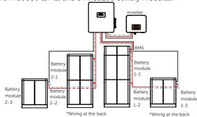
Connect with a MC0600 (BMS) and 8 HV10230 battery modules:
