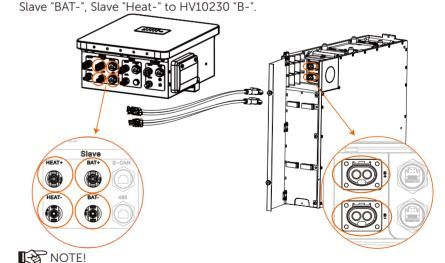
Regardless of how many battery modules installed, please put a waterproof cap on the communication port of the unconnected port of battery module. Please check T-BAT-SYS-HV-3.0 User Manual/Quick installation guide for detailed tutorial on cable-connecting between MC0600 and HV10230 battery modules.
