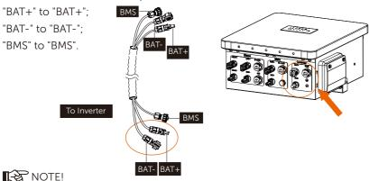
\*It is recommended to protect the cables by using corrugated pipe.
