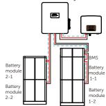
Connect with a MC0600 (BMS) and 6 HV10230 battery modules:
