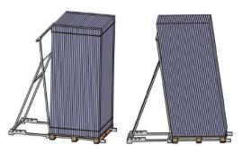
(5) Cut the inner packing belt and lean the modules against a sturdy support or wall.
