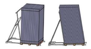
(4) Cut the inner packing belt and lean the modules against a sturdy support or wall.
