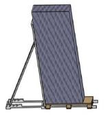
(5) Wear gloves and take out the modules gradually. Two people take out the modules from both sides simultaneously. We suggest that once the modules are unpacked, they should be taken out at one time.
