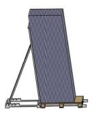
⑥ Wear gloves and take out the modules gradually. Two people take out the modules from both sides simultaneously. We suggest that once the modules are unpacked, they should be taken out at one time.
