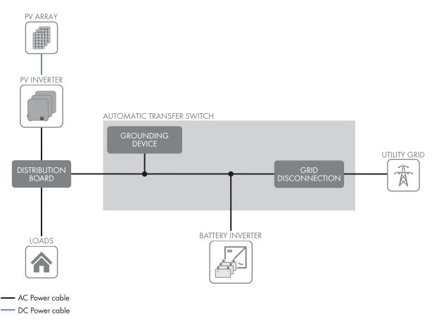
Figure 1: Overview of a single-phase battery-backup system
