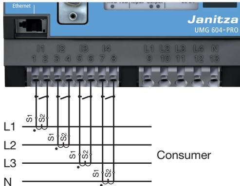
Fig. Current measurement via current transformers connection example.
