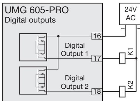
Fig. Connection of an AC voltage relay to the digital outputs.
