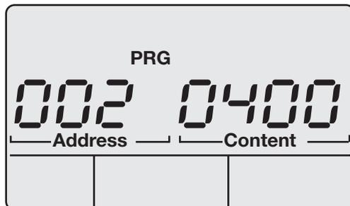
Fig. Example; voltage transformer (primary) for the baseline measurement, address 002 with a content of "400".
