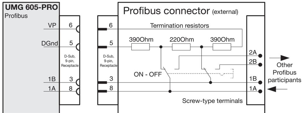
Fig. Profibus connector with termination resistors.
