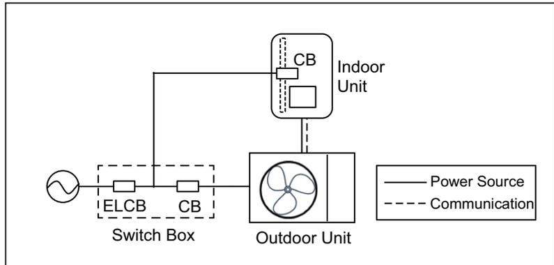
[Power Supply for DHW Boost Heater]
