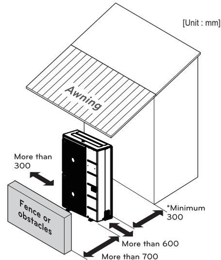
\* Please secure the space, considering field installation of the shut-off valve and strainer.
