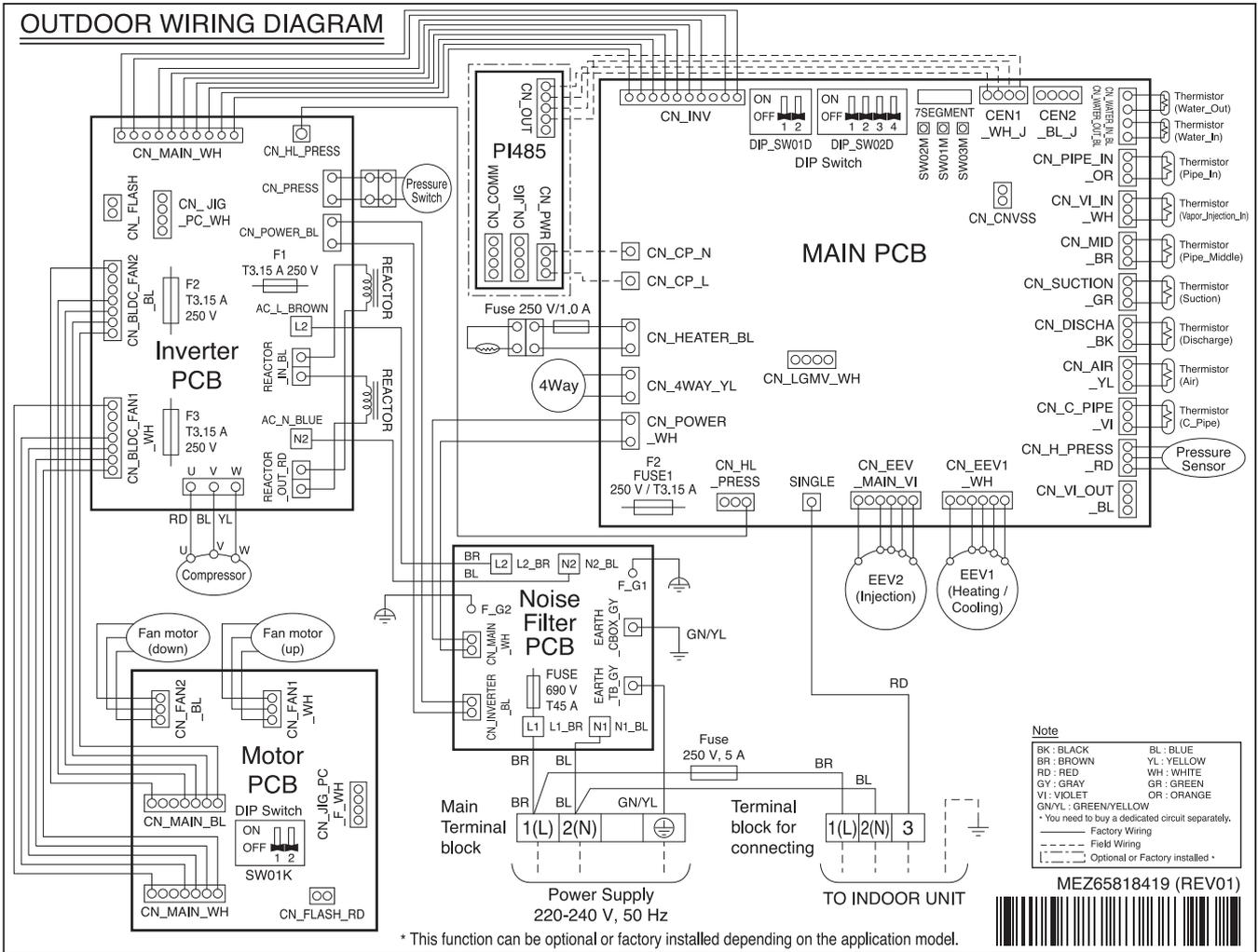
\* This function can be optional or factory installed depending on the application model.
