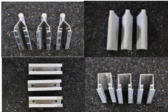
Fig. 10: detail view of test sample after SaltMist
