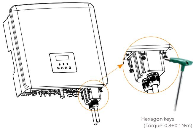
**Step 6.** Tighten the waterproof fastening head.
