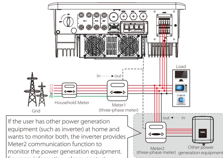
If the user has other power generation equipment (such as inverter) at home and wants to monitor both, the inverter provides Meter2 communication function to monitor the power generation equipment. For more information, please contact us.
