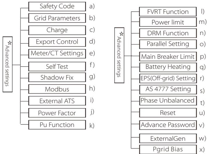
All advanced settings can be set here, such as battery, grid, EPS(Off-grid), etc.
