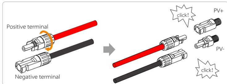
The following is the location of the inverter's positive and negative (PV-/PV+) ports.
