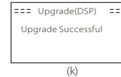
**Step 7.** Plug off the U disk, press "Esc" to return to the main interface, and long press the enter key to exit the mode.
