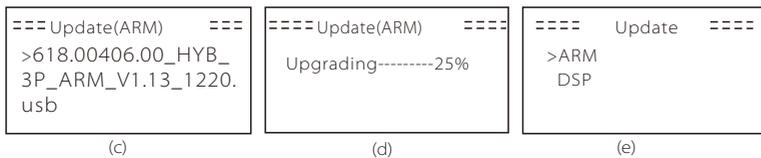
**Step 5.** For DSP: Please wait for 10 seconds. When "Update" page shown as below, press down to select "DSP" and then press Enter. Please confirm the firmware version again and press Enter to upgrade. The upgrade takes about 2 minutes.
