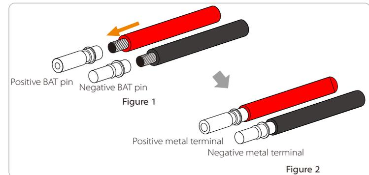
**Step 4.** Tighten the BAT pin needle and the wiring harness to make the connection tight without looseness.
