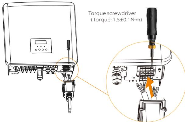
**Step 5.** Install the AC waterproof cover, and tighten the screws on the four sides of the waterproof cover with an Hexagon keys. (Torque:  $0.4\pm 0.1\text{N}\cdot\text{m}$ )
