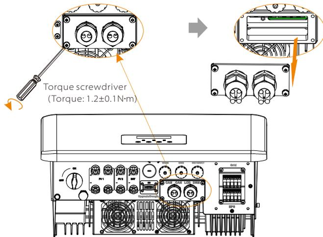
**Step 3.** Insert the communication cable through the communication adapter, and peel off the outer insulation layer of 15 mm.
