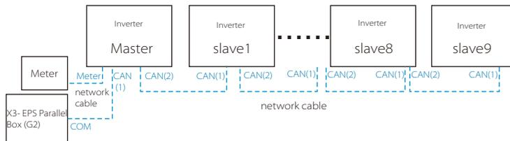
Note:A CT can be used in the parallel connection of the Hybrid series inverters only when the master inverter are with PV panels or only the meter can be used. In the parallel connection of the Fit series inverters, only the meter can be used.
