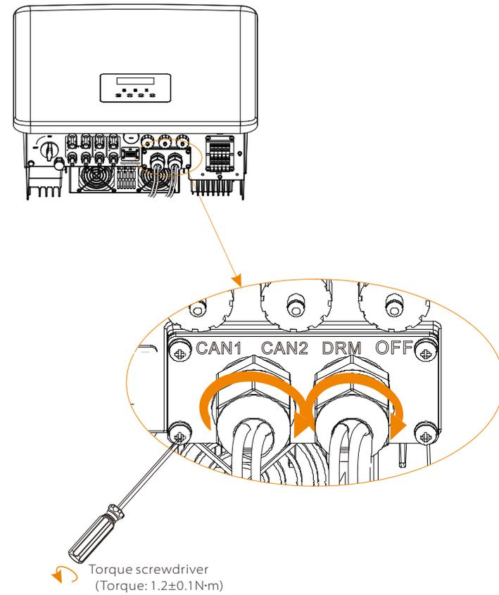
**Step 7:** Finally, find the corresponding COM, BMS, Meter, CT, CAN, DRM, OFF ports on the inverter and insert the communication cable into the corresponding ports.
