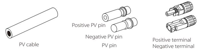
**Step 2.** Use a wire stripper to strip the 7mm insulation layer of the wire end.
