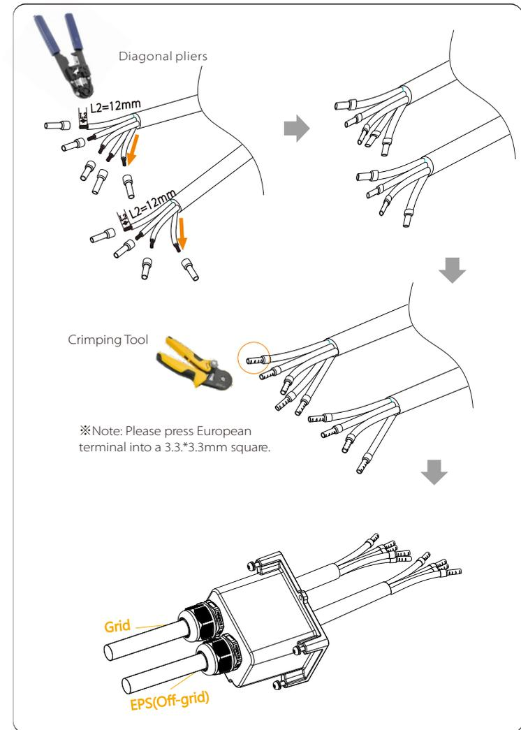
**Step 4.** Find the location of the AC interface on the inverter, insert the crimped terminals into the UW10 terminals L1, L2,L3,N, and PE according to the wire sequence, and use a flat-blade screwdriver to tighten the screws. (Torque:  $1.5\pm 0.1\text{N}\cdot\text{m}$ )
