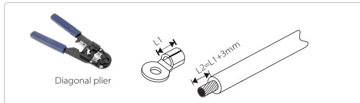
**Step 3.** Insert the striped cable into OT terminal and tighten the terminal with a terminal crimping tool.
