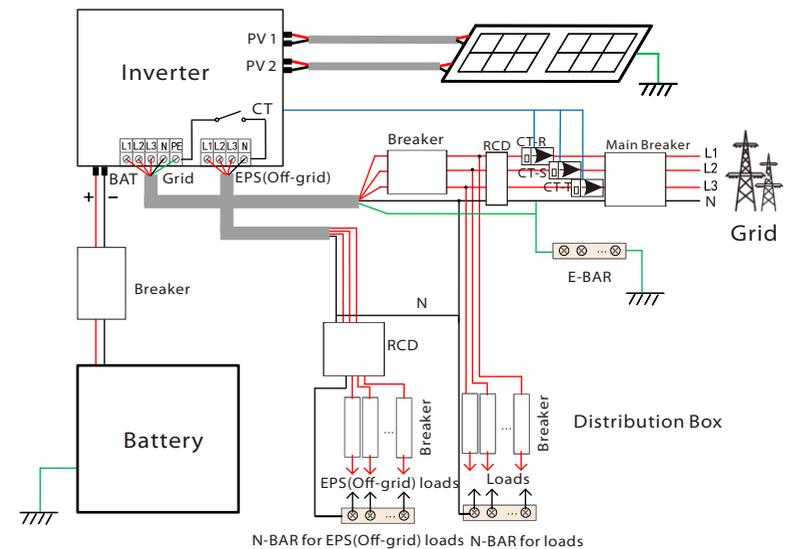
Diagram D: N line and PE line together, M series inverter;
