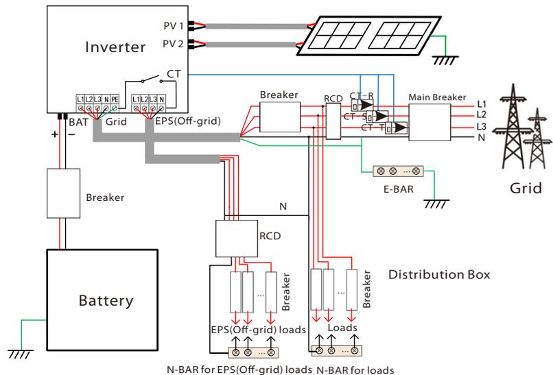
Diagram D: N line and PE line together, all load connection EPS(Off-grid)
