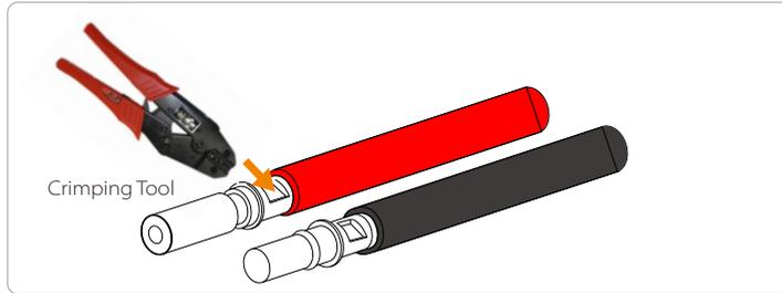
**Step 5.** The PV joint is divided into 2 parts - the plug and the fastening head. Insert the cable through the fastening head and the opposite plug. Note that the red and black lines correspond to different of plugs. Finally, force the cable pair into the plug, will a "click" sound, which indicates that the connection is complete.
