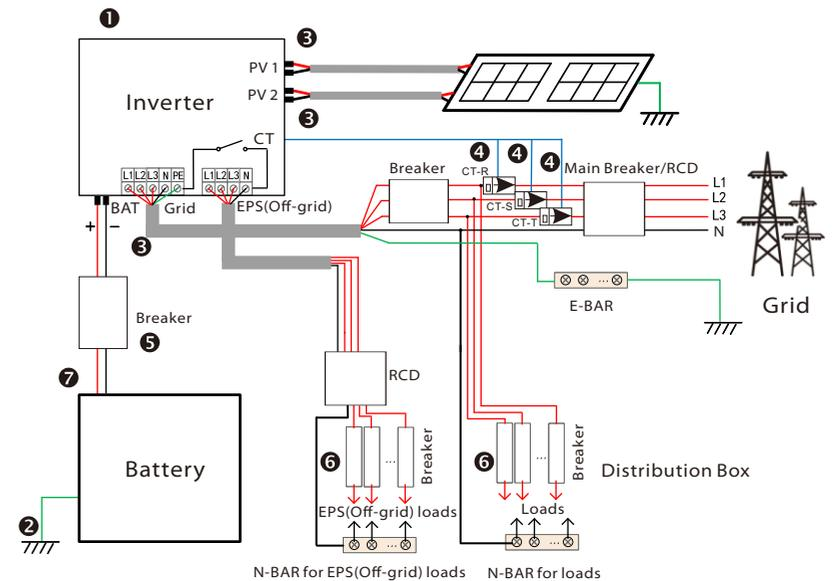
Note: The RCD on the figure represents a leakage protection device with a circuit breaker function.
