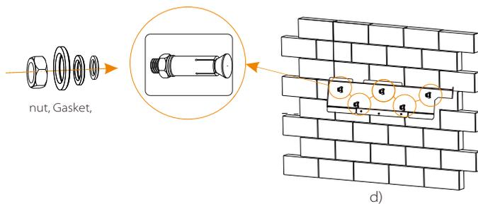
➤ Step 3: Tighten the inverter and bracket
