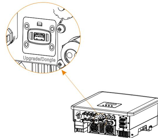
Step 2. Plug Pocket WiFi into the DONGLE port.
