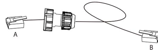
2) One side of the finished cable, Waterproof connector with RJ45 is inserted into the inverter, and one side of the RJ45 terminal is inserted into the CT connection.
