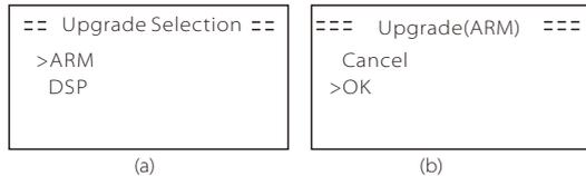
**Step 4.** Please confirm the new firmware version again and select the firmware to upgrade. The upgrade takes about 20 seconds. (d) When it is completed, the LCD screen returns to the "Update" page.
