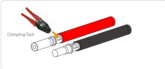
**Step 5.** The BAT joint is divided into 2 parts - the plug and the fastening head. Insert the cable through the fastening head and the opposite plug. Note that the red and black lines correspond to different of plugs. Finally, force the cable pair into the plug, will a "click" sound ,which indicates that the connection is complete.
