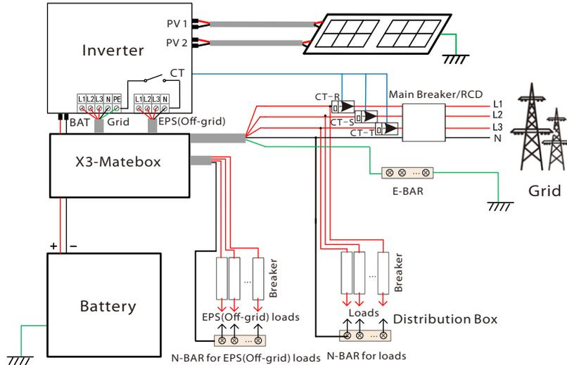
Diagram C: N line and PE line together, D series inverters;
