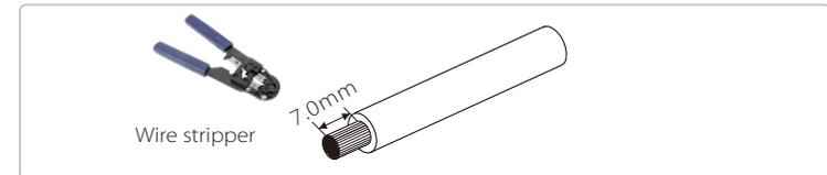
**Step 3.** Tighten the cable with the insulation layer stripped and insert it into the metal terminal (see Figure 1), make sure all wires are inserted into the metal terminal (see Figure 2).
