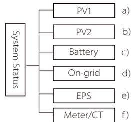
System status contains six content: PV1/PV2/Battery/On-grid (energy feed into or buy from the grid)and EPS(Off-grid) and so on. Press up and down to select, press "Enter" to confirm the selection, and press "ESC" to return to the menu.
