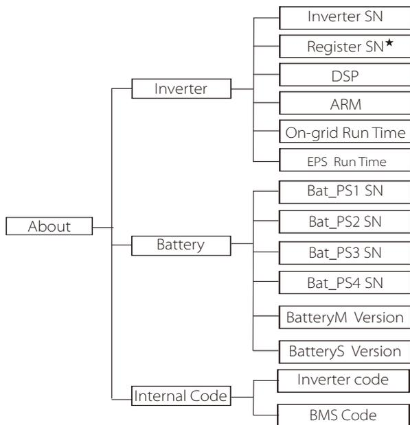
★ Register1 SN: Represents the serial number of external monitoring equipment, such as Pocket WiFi, Pocket LAN.
