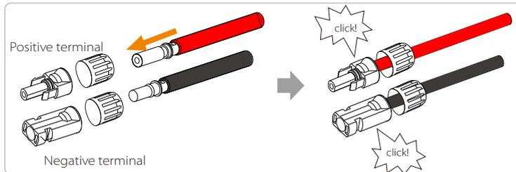
**Step 6.** Tighten the fastening head and into insert the corresponding positive and negative (PV-/PV+) ports of the inverter.
