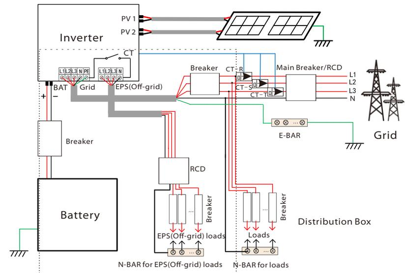
Diagram B: N line and PE line separate wiring, M series inverters;
