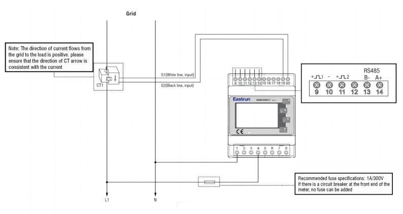
The internal power supply is complete and no external power supply is required.
