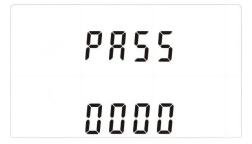
Setting up is password-protected so you must enter the correct password (default '1000') before processing.
