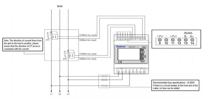
The internal power supply is complete and no external power supply is required.
