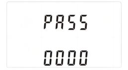
Setting up is password-protected so you must enter the correct password (default '1000') before processing.
