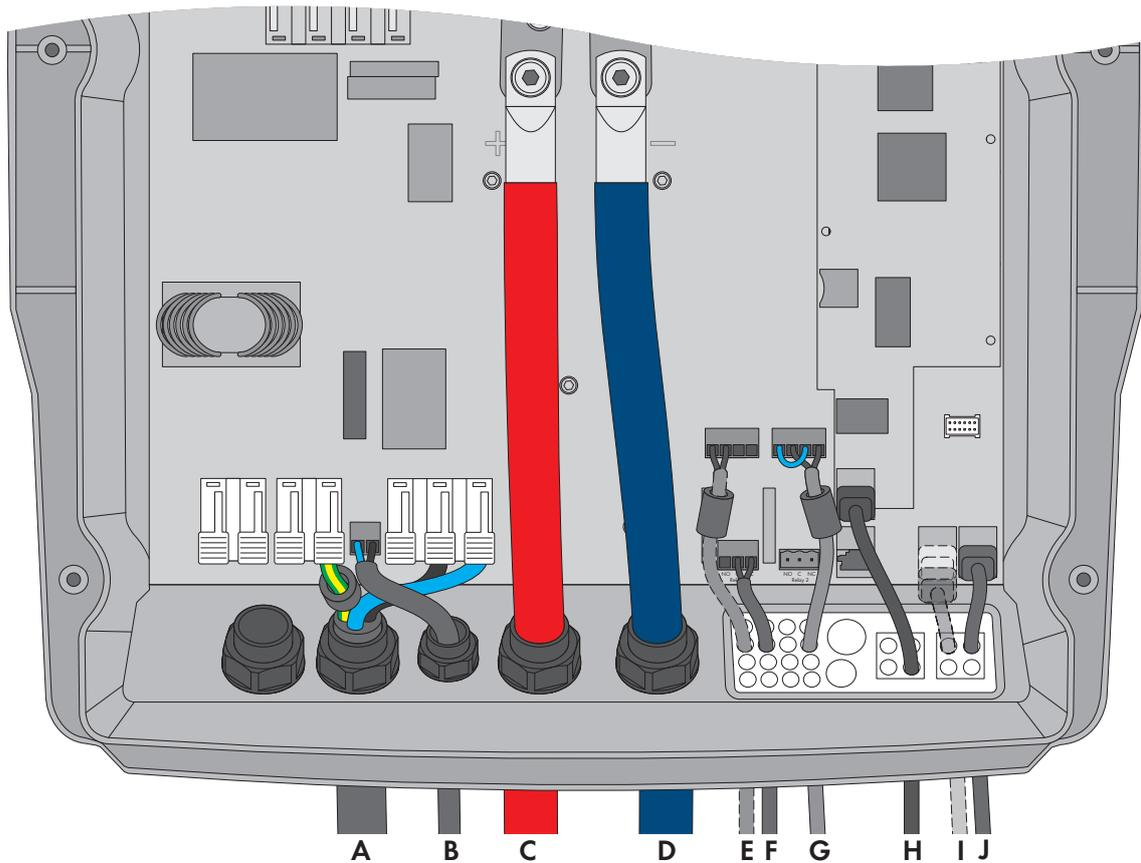
Figure 7: Connecting the master
