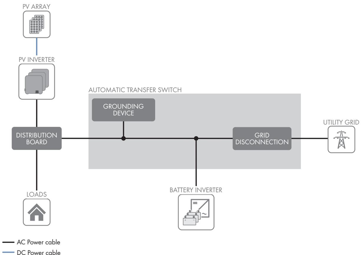
Figure 1: Overview of a single-phase battery-backup system
