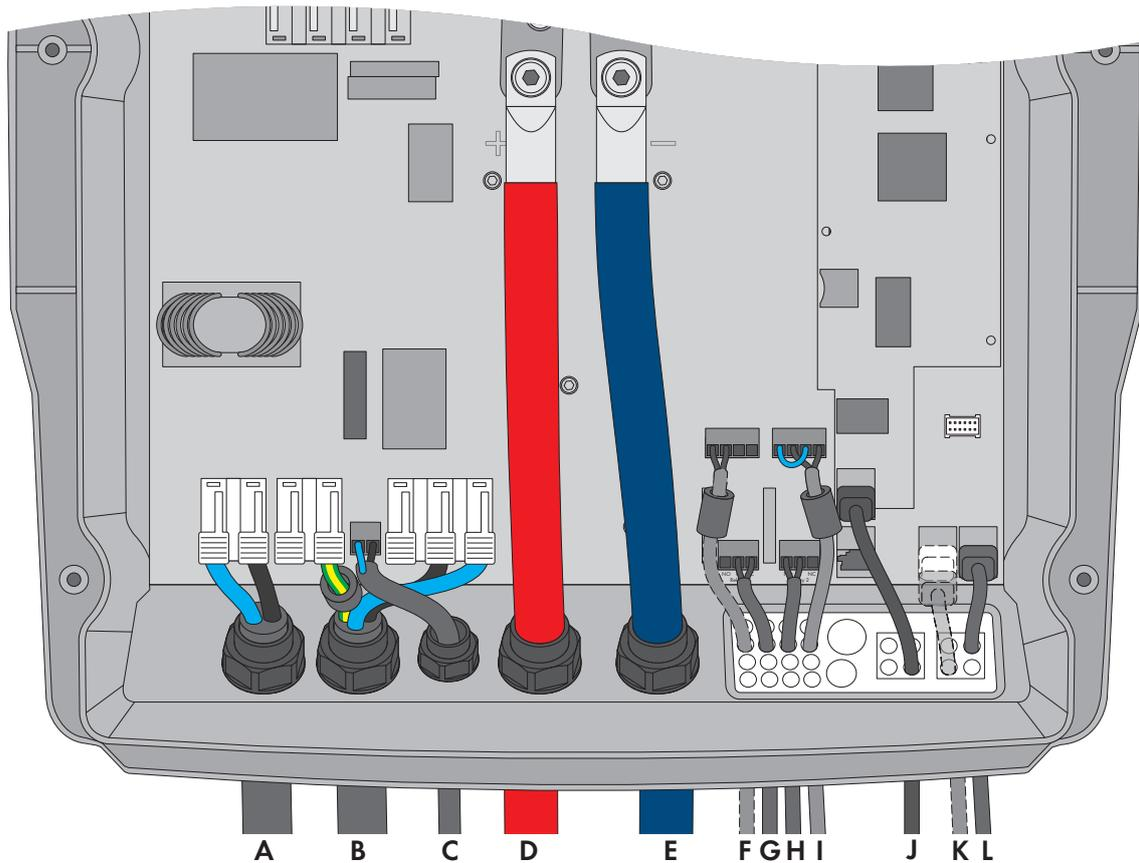
Figure 4: Connecting the master with all-pole disconnection
