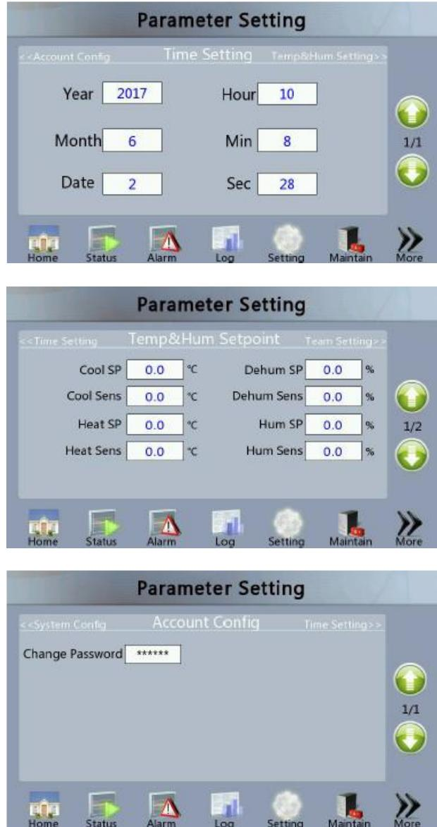
To make the parameter settings: click the corresponding input box, and enter the desired value in the keyboard, as shown in the figure below.
