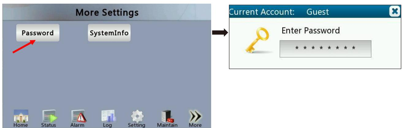
The default password is "0001". The user can change the temperature and humidity set point and temperature and humidity alarm point. Please check the alarm record and alarm history, as well as the system operating state. If the user does not enter the password before entering the parameter, it will automatically jump to the password interface when clicking the corresponding parameter input box.
