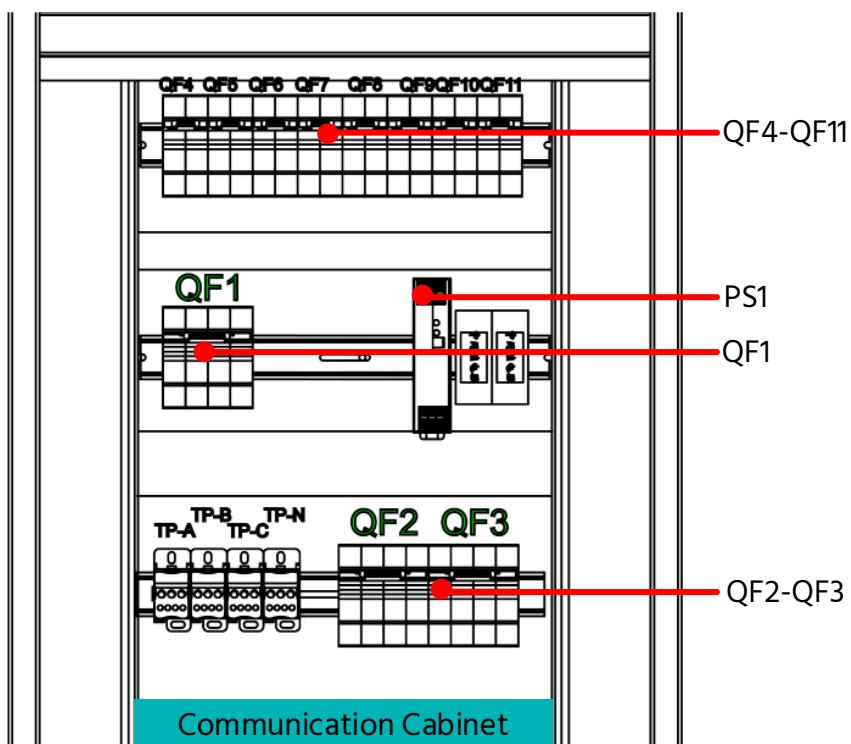
1. Switch on the circuit breaker QF12, and the light of the SPD (Switching Mode Power Supply) will be on.
