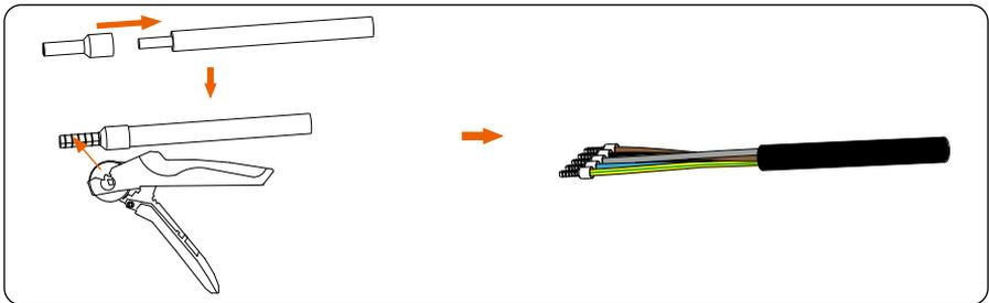
Figure 6-14 Crimp the wires
