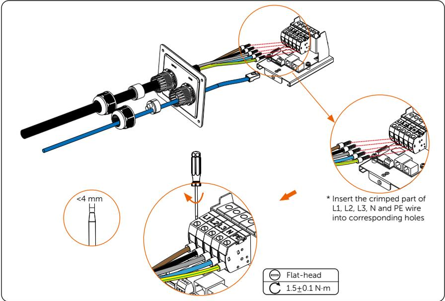
Figure 6-19 Connect the AC input cable
