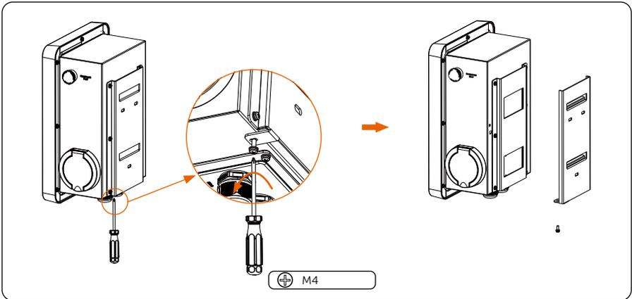
Figure 6-6 Remove the back bracket away
