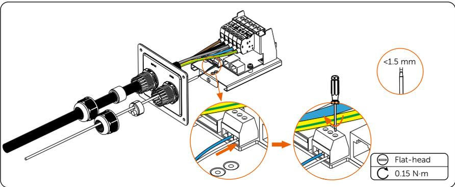
Figure 6-24 Connect the communication cable to RS485 port
