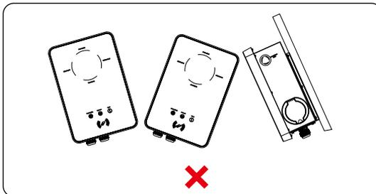
Figure 6-2 Incorrect installation
