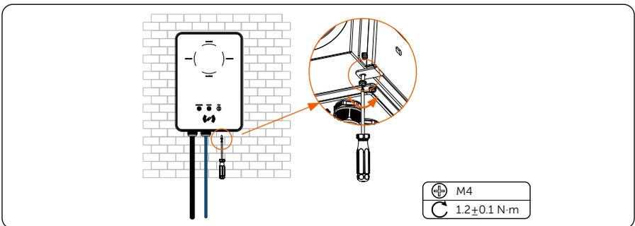
Figure 6-29 Hang and steady the EV-Charger
