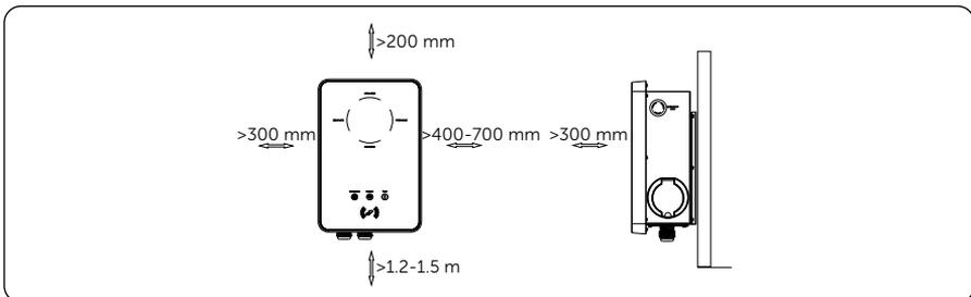
Figure 4-2 Clearance requirement
