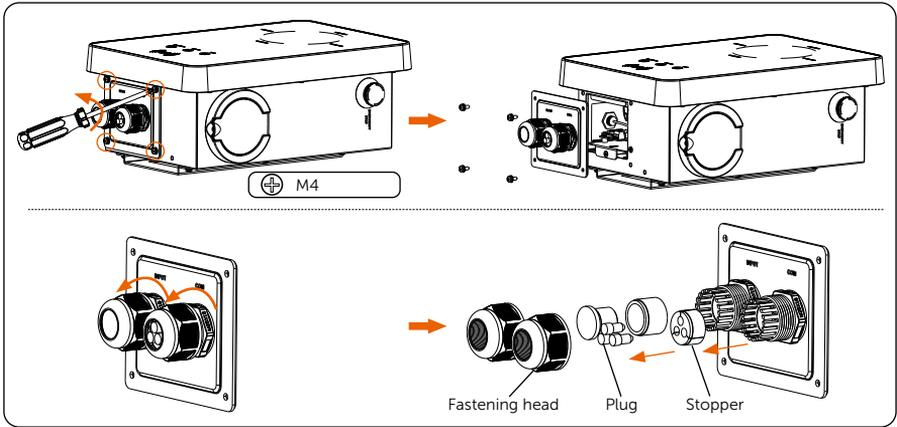
Figure 6-11 Take down and disassemble the rear cover
