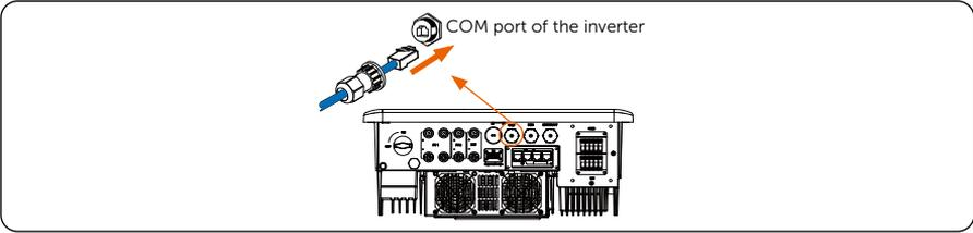
Figure 6-23 Inverter side connection (one example)
