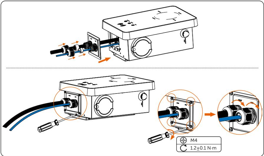
Figure 6-28 Secure the rear cover
