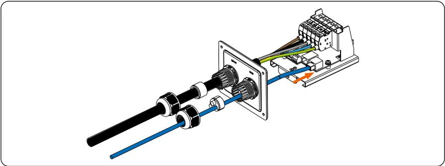
Figure 6-21 Connect the communication cable to RJ45 port
