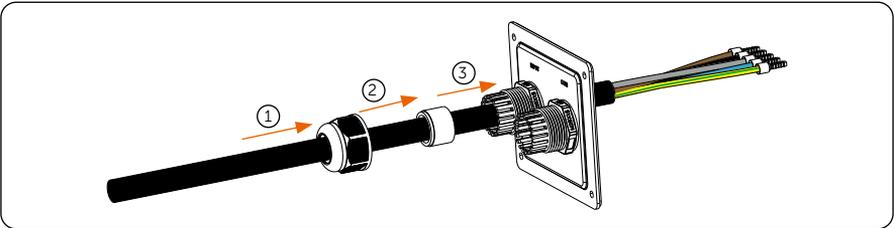
Figure 6-17 Thread the AC input cable
