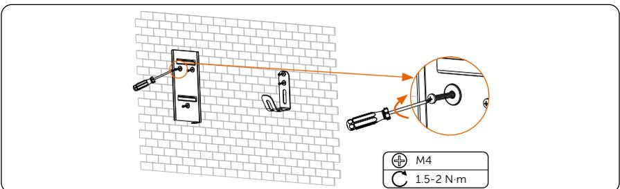
Figure 6-10 Secure the bracket and the cable hook
