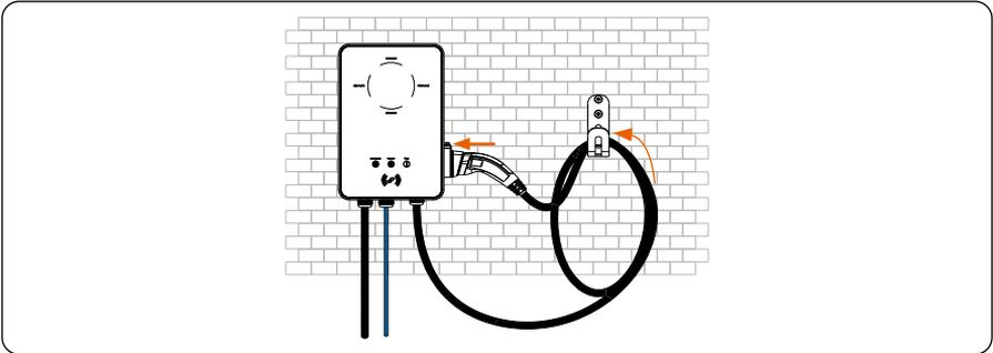
Figure 6-30 Connect the charging connector and hang the cable
