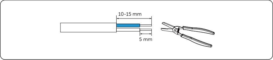
Figure 6-16 Communication cable for connecting Meter
