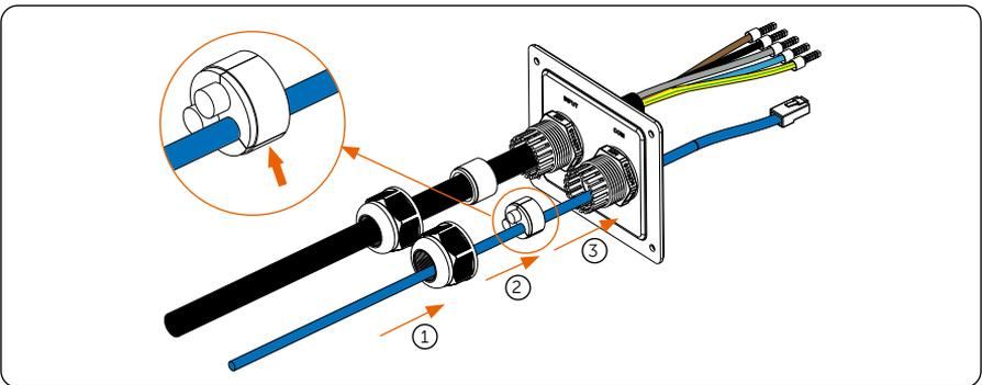
Figure 6-18 Thread the communication cable
