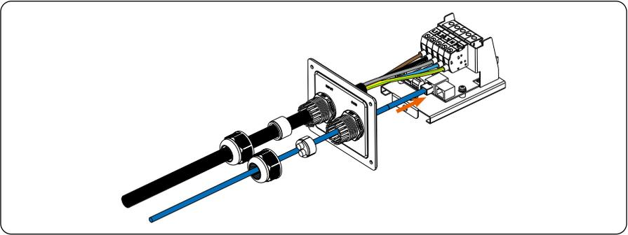
Figure 6-25 Connect the communication cable to Network port
