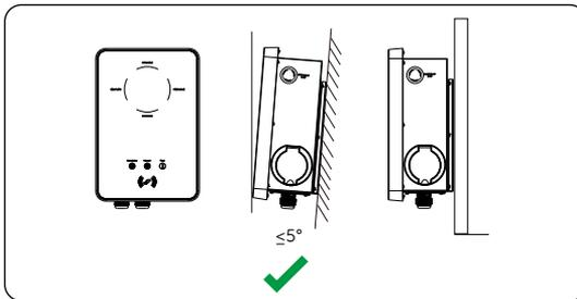
Figure 6-1 Correct installation
