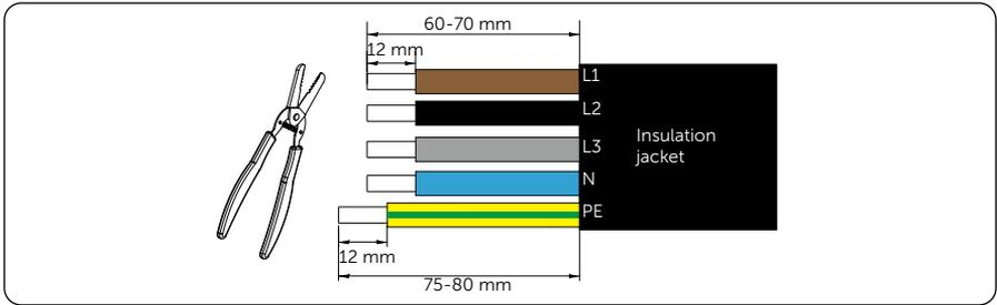
Figure 6-13 Strip the AC input cable
