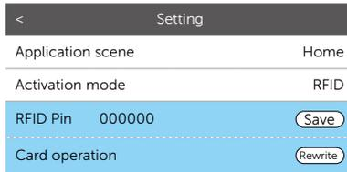
Figure 9-3 Input new RFID Pin and save
