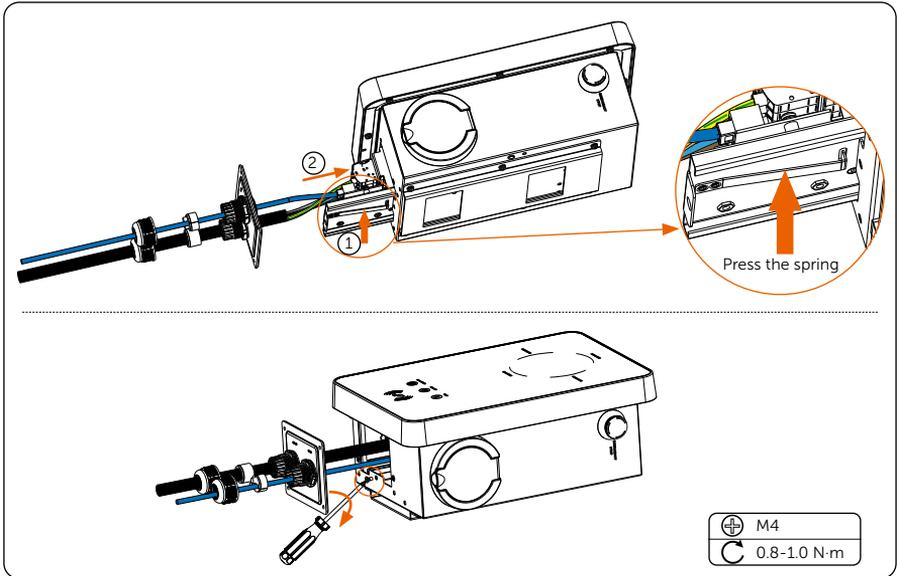
Figure 6-27 Screw the the base plate of communication board
