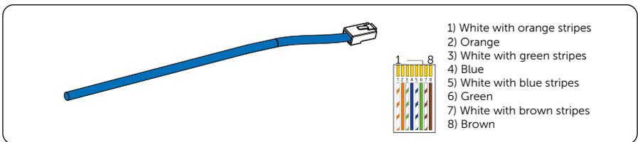
Figure 6-15 Communication cable for connecting CT/Inverter or Network
