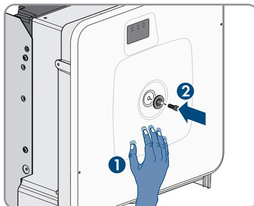
14. Place the cover on the screw in the cover of the enclosure.
