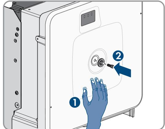
4. Place the cover on the screw in the enclosure lid.
