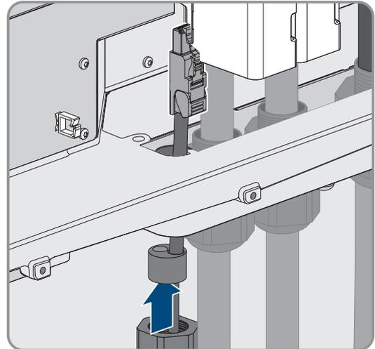
9. When using self-assembly cables, assemble the RJ45 connectors and connect them to the cable.
