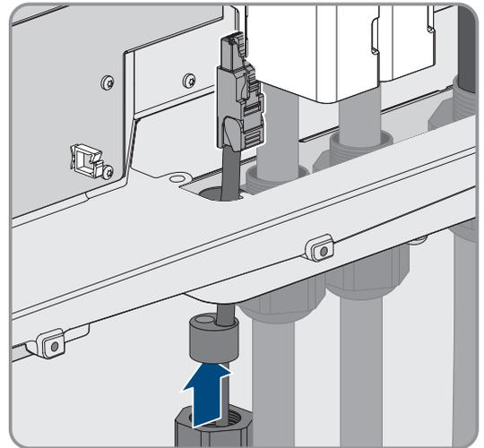
8. When using self-assembly cables, assemble the RJ45 connectors and connect them to the cable (refer to the documentation of the connector).
