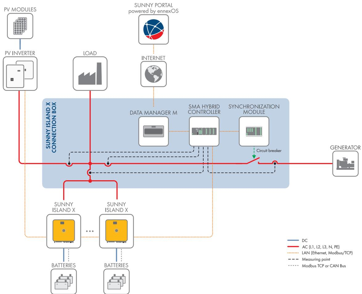
Figure 4: SMA Hybrid Controller as System Manager in a system with a generator (example)
