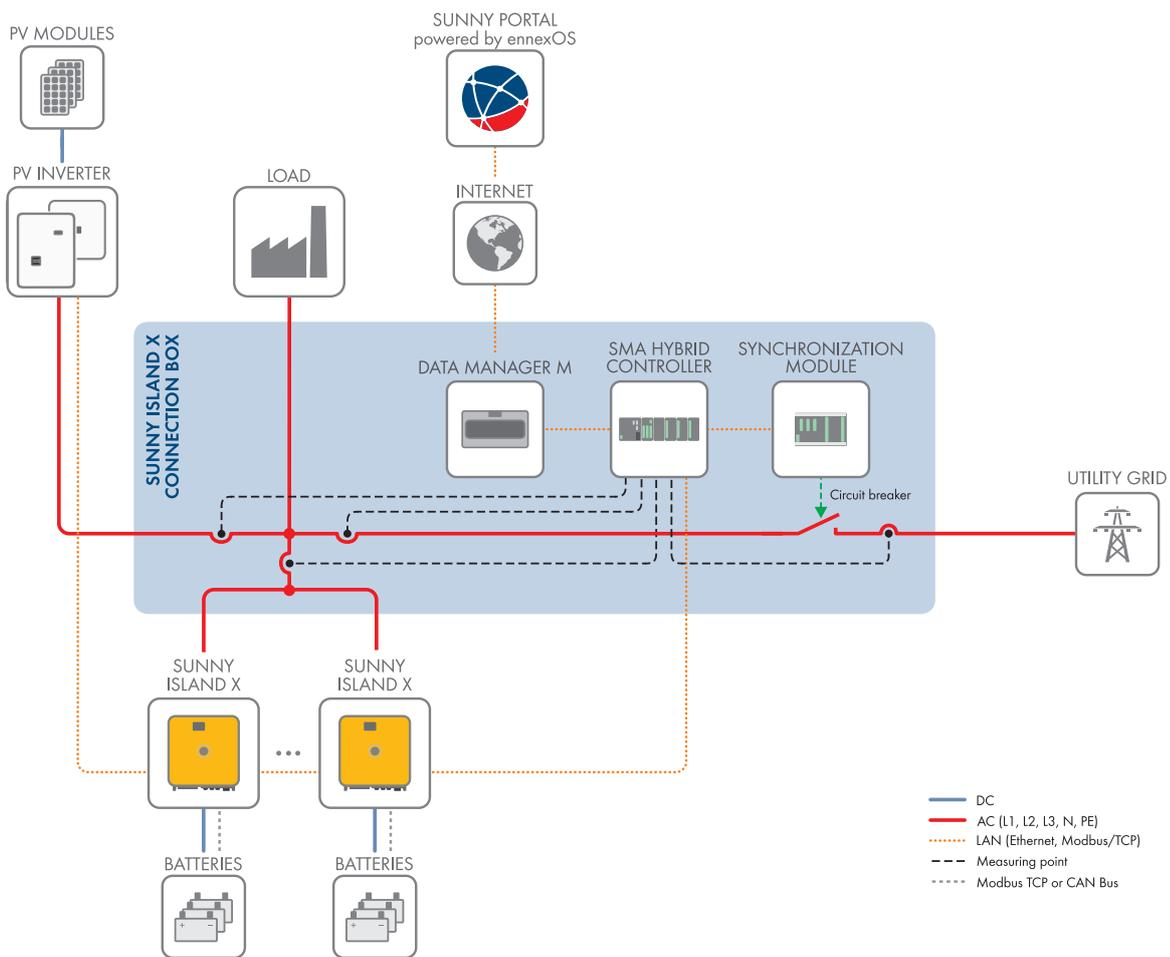
Figure 5: SMA Hybrid Controller as System Manager in a system with utility grid (example)
