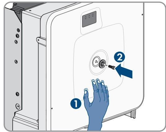
11. Place the cover on the screw in the cover of the enclosure (see Section 13.2, page 104).
