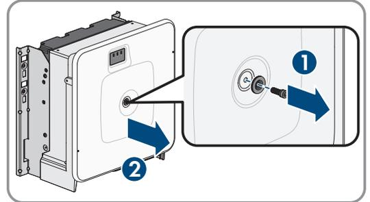
10. Set the screw, cover and cover of the enclosure aside and store safely.
