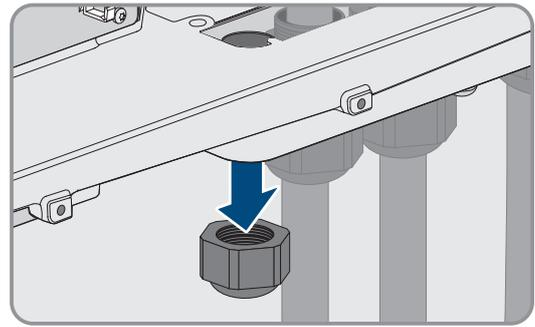
4. Thread the swivel nut over the data cable of the battery.
