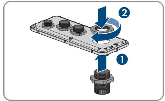
9. Lead the cables through the cable glands in the connecting plate and align the connecting plate by means of the mounting template.
