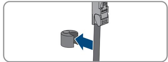
8. Press the cable support sleeve into the 2-hole cable gland and guide the battery data cable to the socket **BAT ETH**. Lay the battery data cable according to the installation plan and attach it to the brackets.
