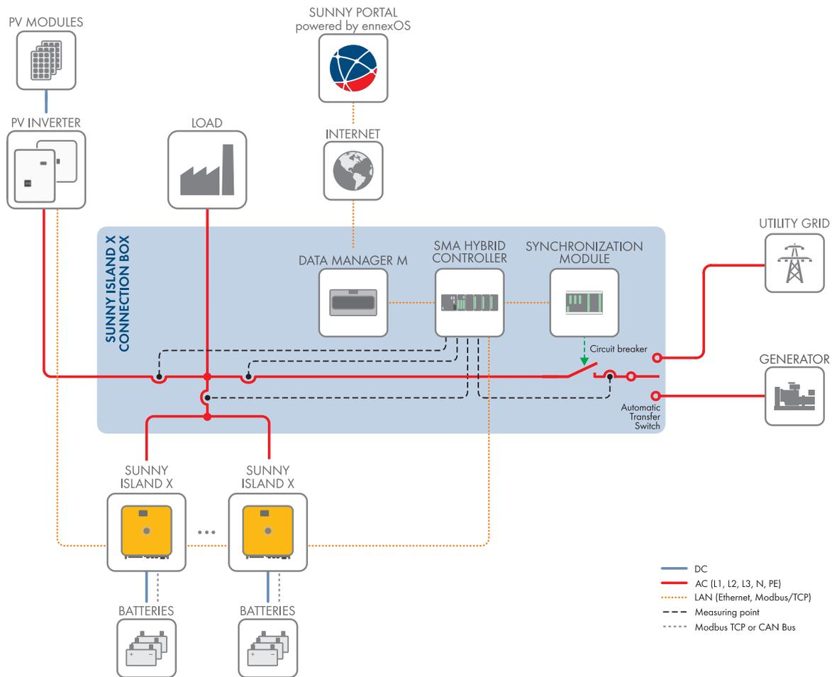
Figure 6: SMA Hybrid Controller as System Manager in a system with utility grid and generator (example)
