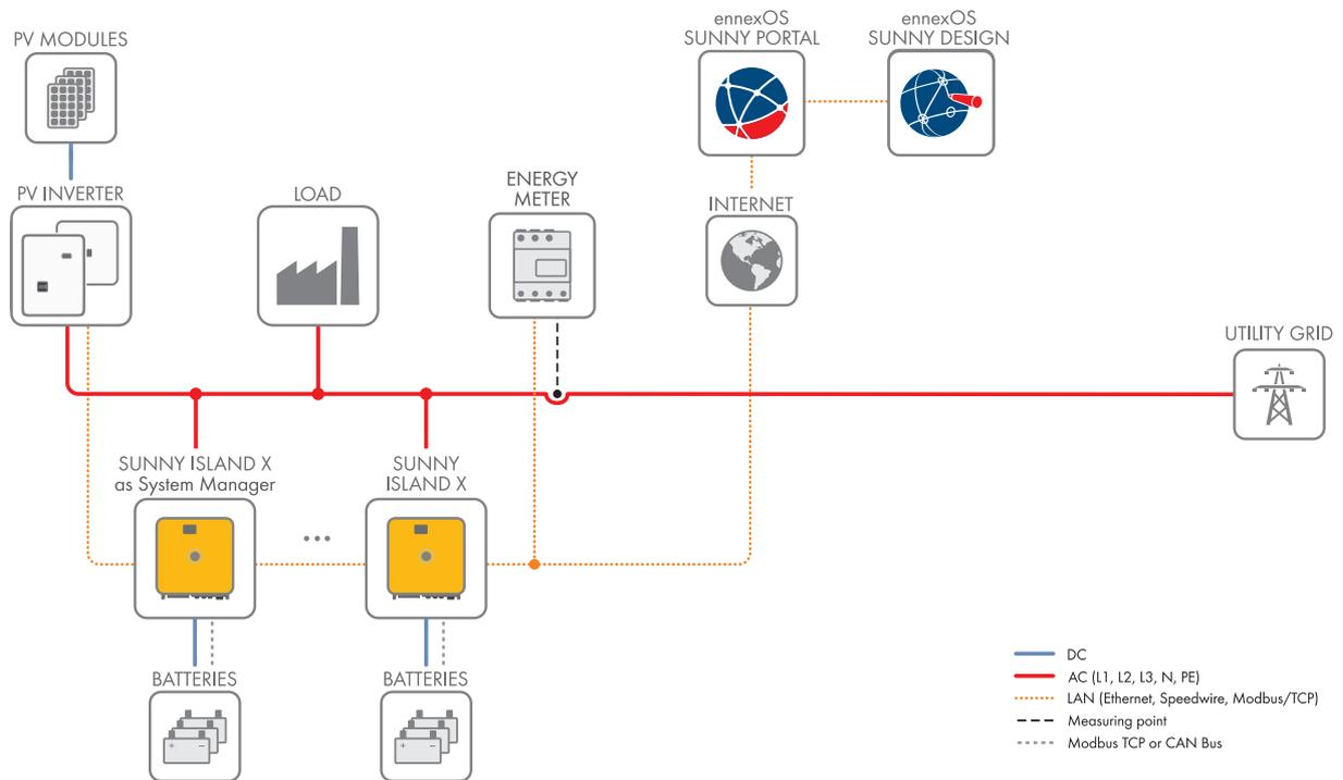
Figure 2: Sunny Island X as System Manager in a system with utility grid (example)
