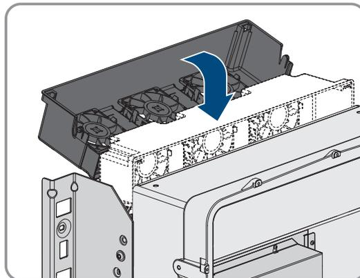
7. Guide the fan bracket on the enclosure vertically downwards into the enclosure brackets provided.
