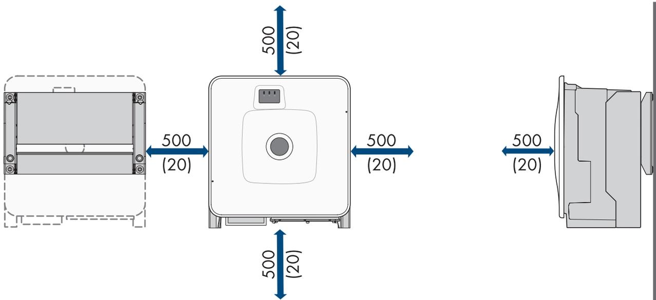
Figure 12: Recommended clearances (dimensions in mm (in))
