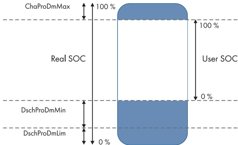
Figure 9: State of charge ranges of the battery
