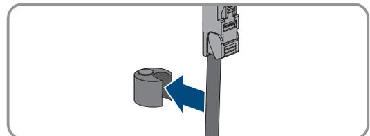
8. Press the two-hole cable support sleeve into the cable gland and guide the battery communication cable to the socket **BAT CAN**. Lay the battery data cable according to the installation plan and attach it to the brackets.
