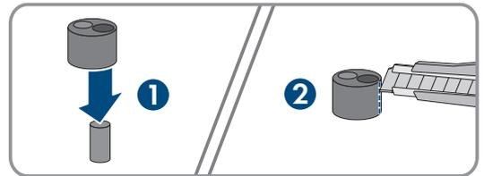
6. Insert each network cable into a 2-hole cable support sleeve.
