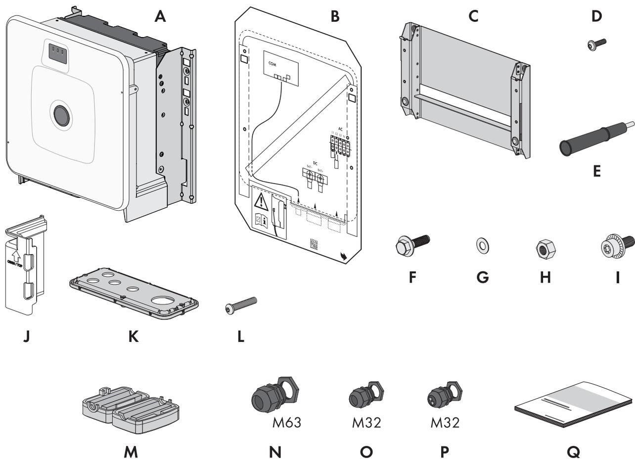
Figure 1: Components included in scope of delivery
