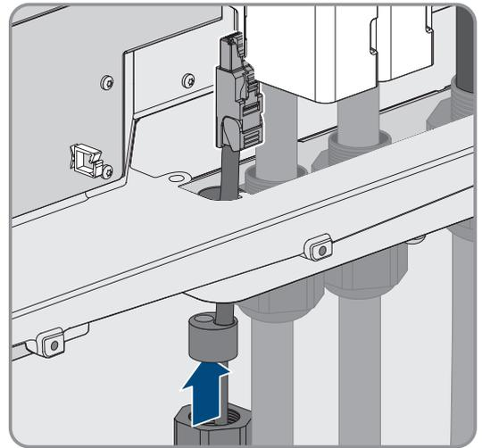
9. When using self-assembly cables: Assemble the RJ45 connectors according to the specified pin assignment and connect them to the cable.
