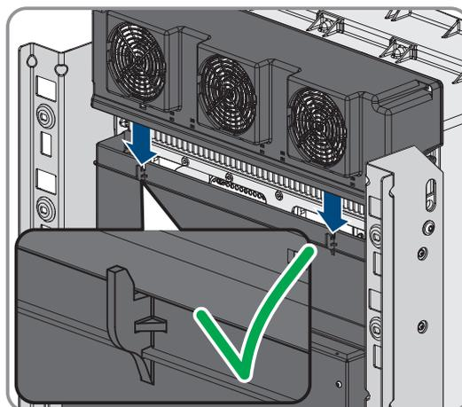
8. Press the fan bracket firmly downwards so that the locking tabs engage on the right and left.
