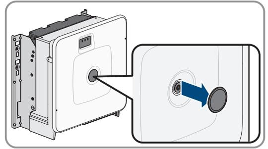
9. Unscrew the screw on the enclosure lid (hex socket, AF8) and remove the enclosure lid.
