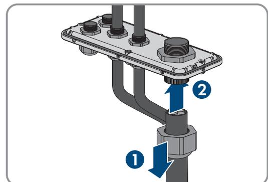
8. Attach the cable glands to the connecting plate.
