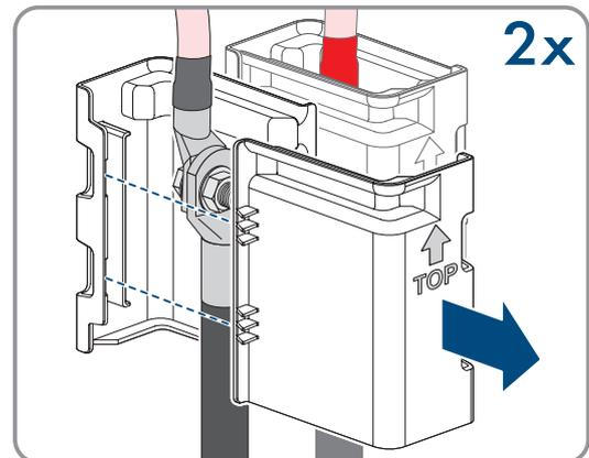
4. Remove the DC cable connection. Loosen the hex nuts (AF10) and remove the combined hexagon head screw (AF16).
