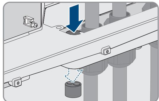
5. For each network cable, remove one of the plugs from the enclosure openings and for each network cable cut an enclosure opening with a utility knife.
