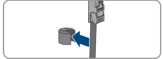
7. Press the 2-hole cable support sleeve into the cable gland and guide each network cable to the network port. Lay each cable according to the installation plan and attach it to the brackets.
