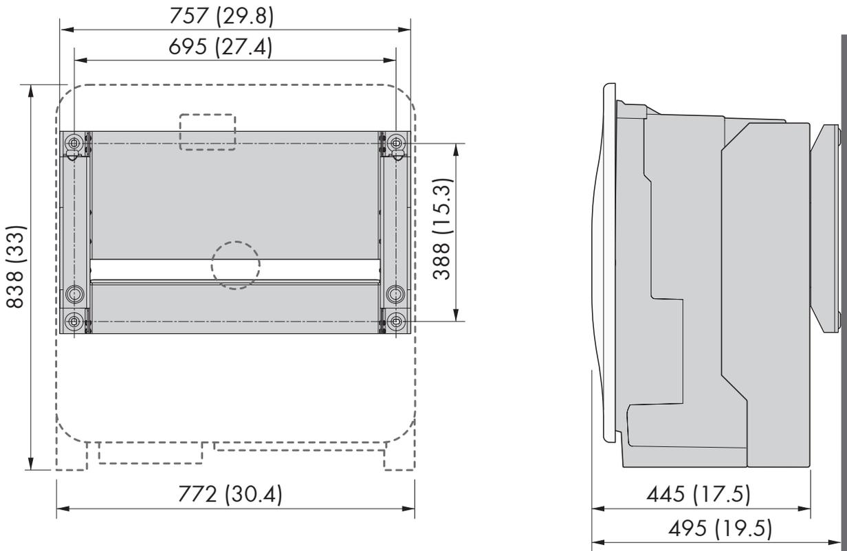
Figure 11: Position of the anchoring points (dimensions in mm (in))
