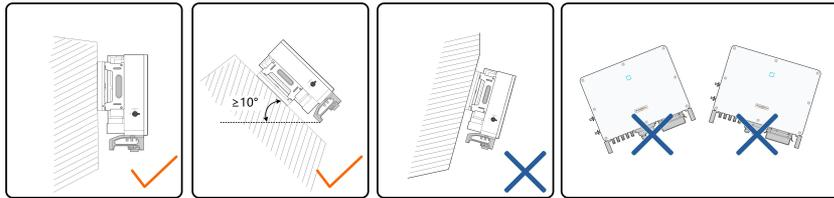
In case the installation site is a level surface, mount the inverter to the bracket to meet the mounting angle requirements, as shown in the figure below.
