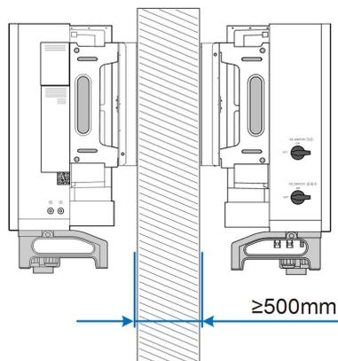
Install the inverter at an appropriate height for ease of viewing LED indicator and operating switch(es).
