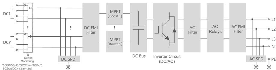
figure 2-4 Circuit Diagram
