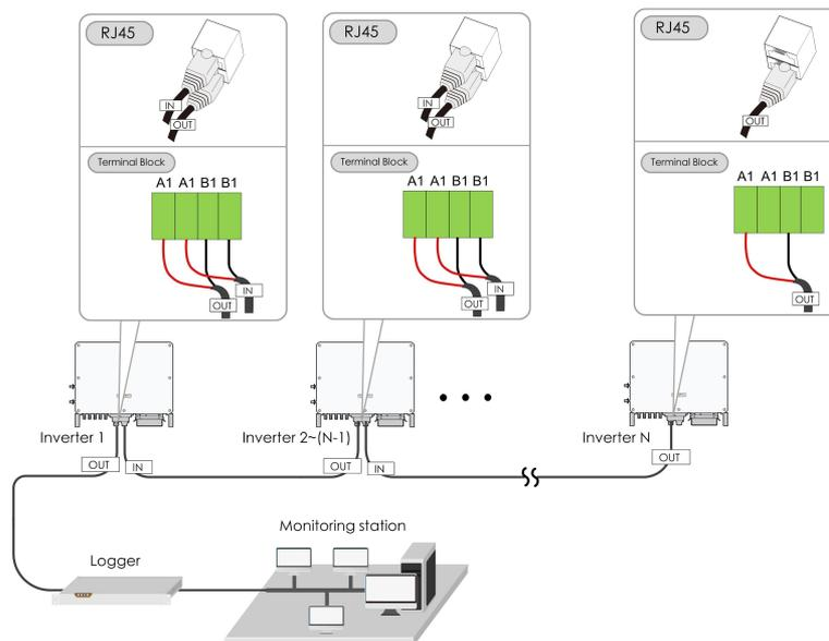
figure 5-5 Multi-inverter Connection
