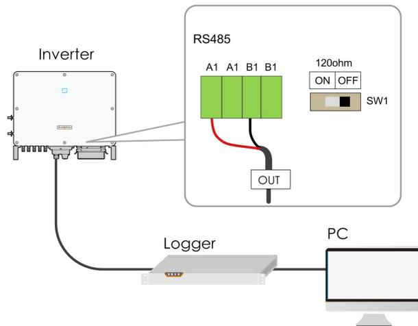
figure 5-4 Single-inverter Connection
