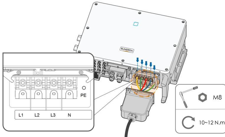
Ensure that the depth L of the socket used is not less than 18mm.
