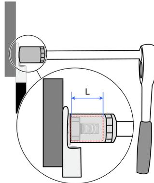
step 7 Secure the junction box, fasten the buckle, and secure it with supplied M4×10 screw.
