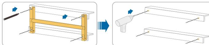
step 3 Secure the mounting-bracket with bolts.
