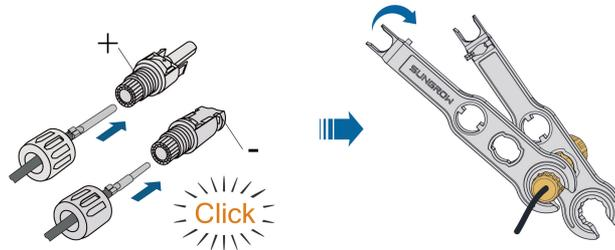
step 4 Check for polarity correctness.
