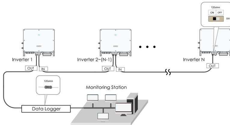
figure 5-6 Configuration of Dip Switch ( $N \geq 15$ )
