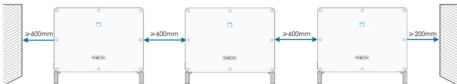
In case of back-to-back installation, reserve specific clearance between the two inverters.
