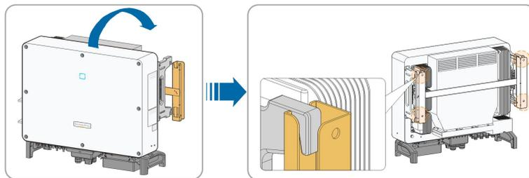
step 4 Fix the inverter with screws.
