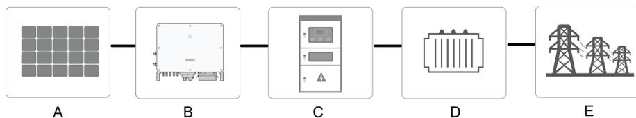
figure 2-1 Inverter Application in PV Power System
