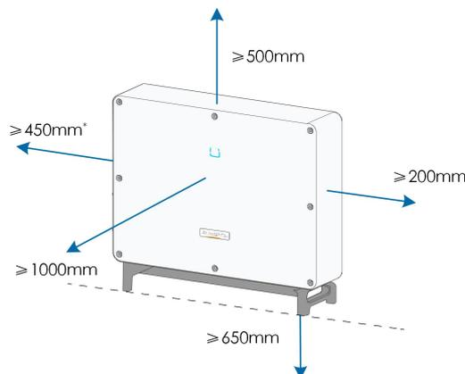
\* In case this distance is less than the distance in the diagram, move the inverter from the mounting-bracket or wall before maintaining fans.
