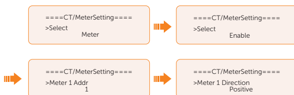
Figure 14-13 Setting meter for the inverter
