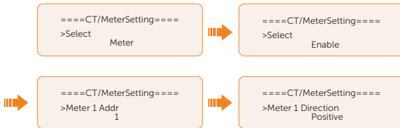
Figure 14-18 Setting meter for the inverter
