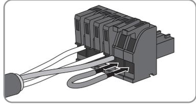
8. Plug the six-pole plug into the port **X2** on the product.
