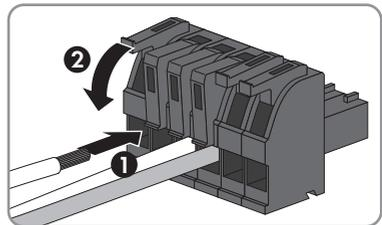
7. If the product is at the end of the RS485 bus, install a jumper wire as a line terminator between pin **5** and pin **6** on the six-pole plug.
