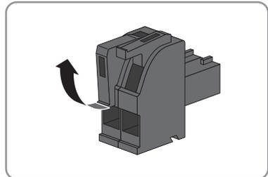
4. Connect the connection cable to the supplied two-pole plug. To do so, plug the conductors into the conductor entries and close the conductor entries. Observe the plug assignment.
