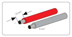
Figure 8-30 Stripping the battery cable
