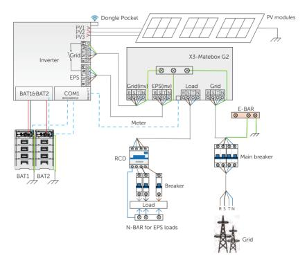
Figure 2-9 Application scheme with a matebox for Australia
