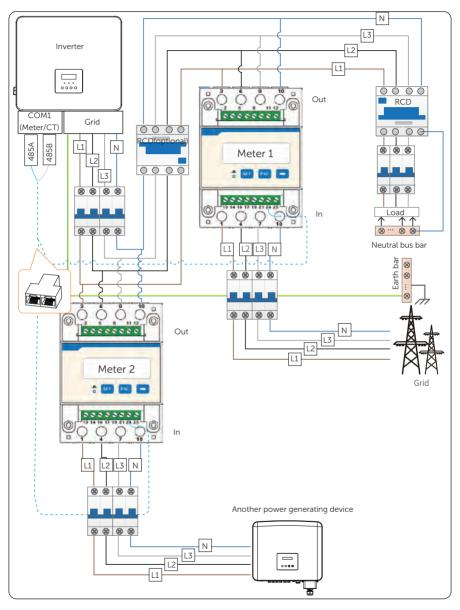
Figure 15-13 Connection diagram of two direct-connected meters
