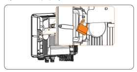
Figure 7-8 Locking the inverter
