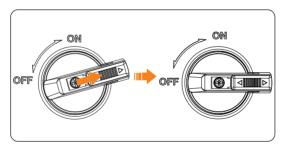
Figure 9-70 Unlocking the DC switch
