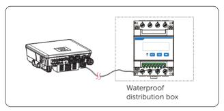
Figure 15-11 Connecting inverter to meter
