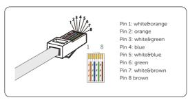
Figure 8-49 Inserting the signal wires and crimping the cable
