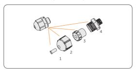
Figure 8-61 Disassembling the waterproof connector
