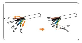
Figure 8-10 Crimping core and ferrule together
