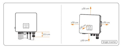
Figure 5-4 Clearance requirement for single inverter
