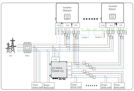
Figure 15-17 With X3-PBOX-150kW-G2 system wiring diagram
