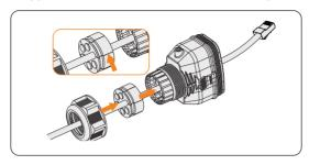
Figure 8-47 Threading the cable with the RJ45 terminal
