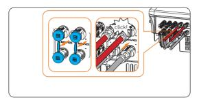
Figure 8-35 Connecting the battery connector
