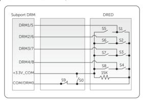
Figure 8-55 DRED connection diagram
