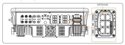
Figure 15-11 Connectiong port for DataHub
