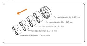
Figure 8-13 Taking out sealing plug
