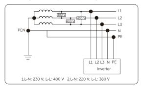
Figure 2-4 Supported power grid-TN-C-S
