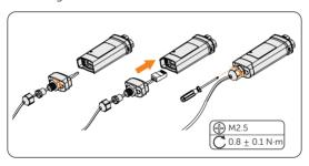
Figure 8-62 Assembling the dongle
