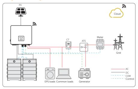
Figure 15-2 Dry contact wiring diagram
