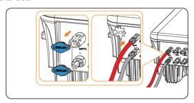
Figure 8-28 Connecting the PV cable
