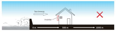
Figure 5-2 Incorrect installation position
