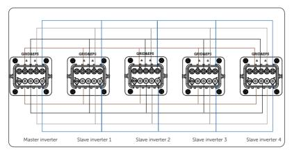
Figure 15-20 Power cable wiring without X3-PBOX-150kW-G2
