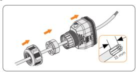
Figure 8-48 Threading the cable without the RJ45 terminal and striping
