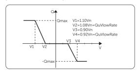
Figure 10-6 Curve Q= f(V)
