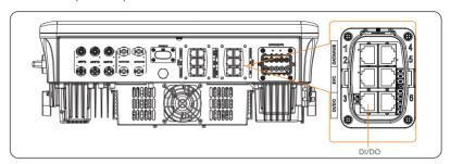
Figure 15-3 Connection port for generator
