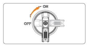
Figure 9-67 Turning on the DC switch
