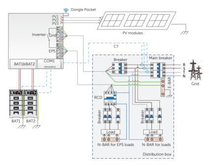
Figure 2-8 Application scheme without a matebox for Australia
