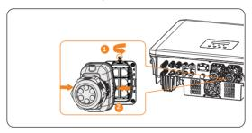
Figure 8-45 Disassembling the COM 2 connector
