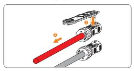
Figure 13-2 Disconnecting the PV connector
