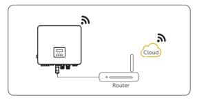
Figure 8-58 LAN mode connection diagram
