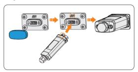
Figure 8-60 Connecting the dongle
