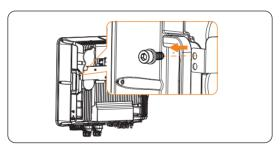
Figure 13-7 Removing the M5 screw
