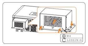
Figure 7-11 Securing the wire shielding cover
