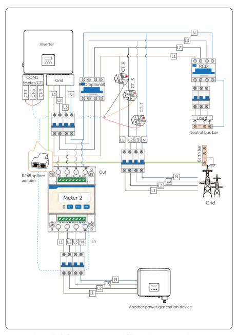
Figure 15-12 Connection diagram of CT and direct-connected meter
