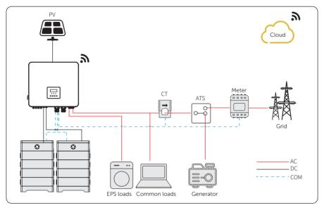
Figure 15-1 ATS control wiring diagram
