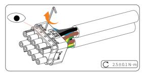
Figure 8-17 Inserting the EPS cable into the rubber core and tightening
