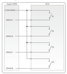
Figure 8-56 RCR connection diagram
