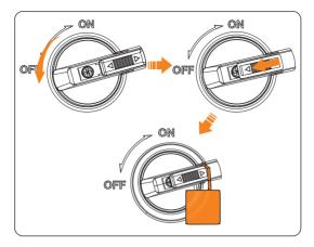
Figure 9-69 Locking the DC switch
