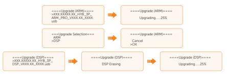
e. After the upgrade is completed, the LCD screen displays Upgrade Successful. If the upgrade fails, the LCD screen displays Upgrade failed.
