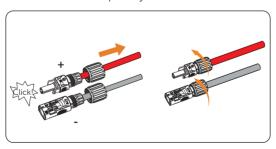
Figure 8-26 Securing the PV cable
