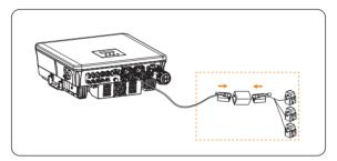
Figure 15-3 Connecting the inverter to the CT
