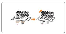
Figure 7-10 Sorting and threading cables
