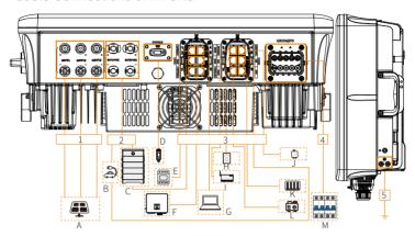
Figure 8-2 Cable connections of inverter
