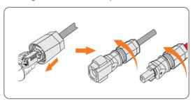
Figure 8-34 Tightening the connector
