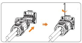
Figure 8-21 Inserting the AC connector into the port and locking it
