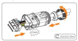
Figure 8-18 Assembling the AC connector
