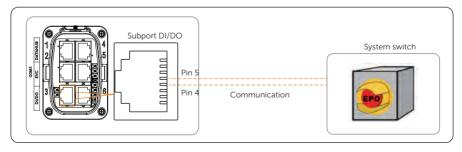
Figure 8-54 System switch connection diagram
