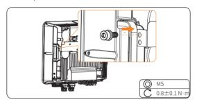
Figure 7-7 Securing the inverter
