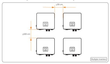
Figure 5-5 Clearance requirement for multiple inverters
