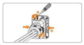
Figure 13-6 Disconnecting the communication connector
