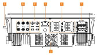
Figure 8-1 Ports and parts of Inverter
