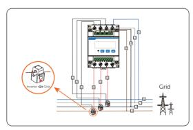
Figure 15-9 Connecting CT-connected meter to the grid
