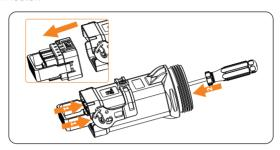
Figure 8-14 Poking the rubber core out
