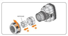
Figure 8-37 Disassembling the connector enclosure
