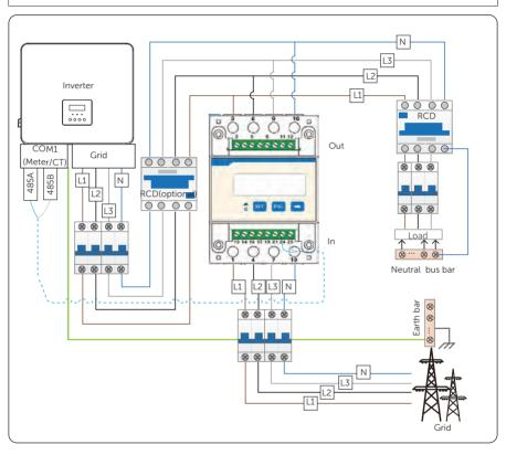
Figure 15-4 System wiring with direct-connected meter
