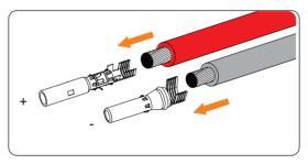
Figure 8-23 Inserting the PV pin contact
