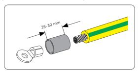
Figure 8-4 Installing the tubing and OT teriminal
