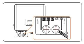
Figure 7-9 Cutting the wire protection ring
