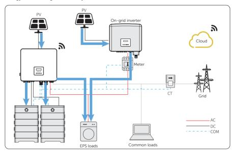
Figure 15-15 Power flowing when grid off
