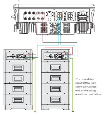
Figure 8-44 BMS connection diagram
