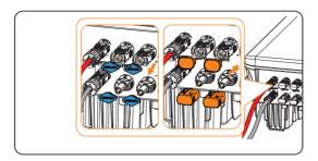
Figure 8-29 Sealing unused ports with buckles
