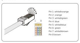
Figure 8-40 Inserting the signal wires and crimping the cable
