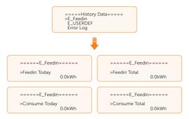
• **E\_USERDEF**: The output electricity of the connected on-grid inverter totay and in total (detected by Meter 2). This function is only available when meter 2 is connected.
