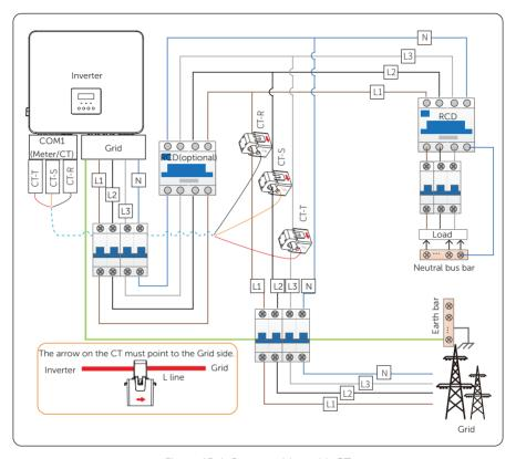
Figure 15-1 System wiring with CT
