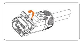
Figure 8-20 Pulling the latch up
