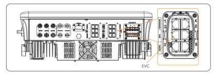
Figure 15-8 Connection port for EV-Charger
