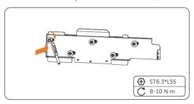
Figure 7-4 Securing the bracket
