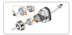
Figure 8-38 Threading the cable with the RJ45 terminal
