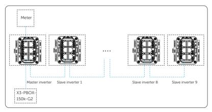
Figure 15-21 Communication wiring with X3-PBOX-150kW-G2
