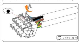
Figure 8-16 Inserting the Grid cable into the rubber core and tightening
