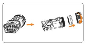
Figure 8-11 Disassembling the AC connector
