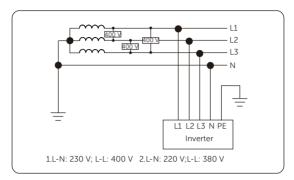
Figure 2-2 Supported power grid-TT
