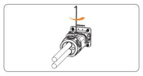
Figure 13-4 Loosening the screw
