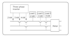
Figure 10-2 Phase Unbalanced enabled
