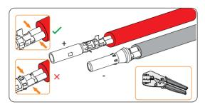
Figure 8-24 Crimping the terminal
