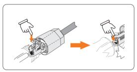
Figure 8-33 Closing the spring
