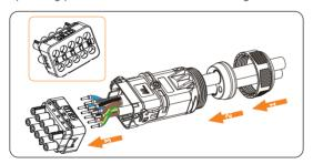
Figure 8-15 Threading and tightening conductors
