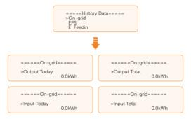
EPS: The output electric energy of the inverter totay and in total, when it is disconnected from the grid (through the EPS port).
