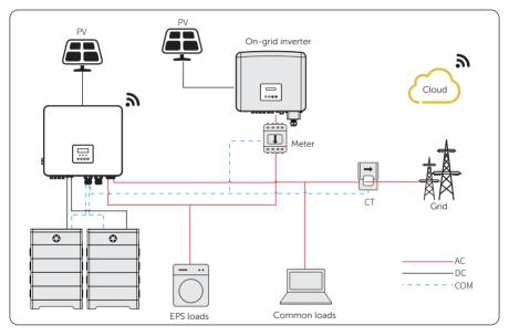
Figure 15-13 Micro-grid wiring connection
