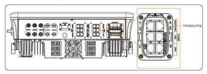
Figure 15-5 Connection port for Adapter Box G2
