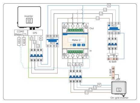
Figure 15-16 Connection diagram of Meter on EPS port
