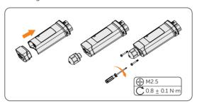
Figure 8-59 Assembling the dongle
