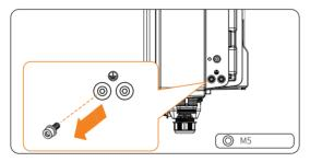
Figure 8-7 Uninstalling the screw
