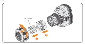
Figure 8-46 Disassembling the connector enclosure
