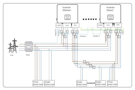
Figure 15-18 Without X3-PBOX-150kW-G2 system wiring diagram
