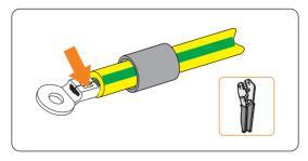
Figure 8-5 Crimping the cable
