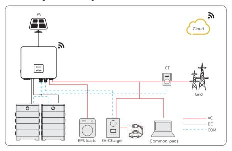
Figure 15-7 EV-Charger wiring diagram
