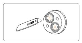
Figure 8-12 Cutting the round membrane
