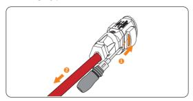
Figure 13-3 Disconnecting the battery connector
