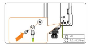
Figure 8-8 Securing the PE cable
