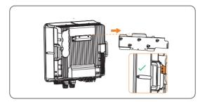
Figure 7-6 Hanging the device onto the bracket
