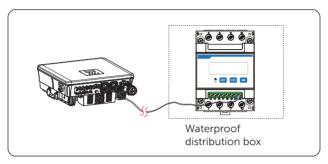
Figure 15-7 Connecting inverter to meter
