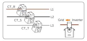
Figure 15-2 Clipping CTs to grid cables
