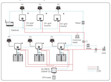
Figure 15-10 DataHub wiring diagram
