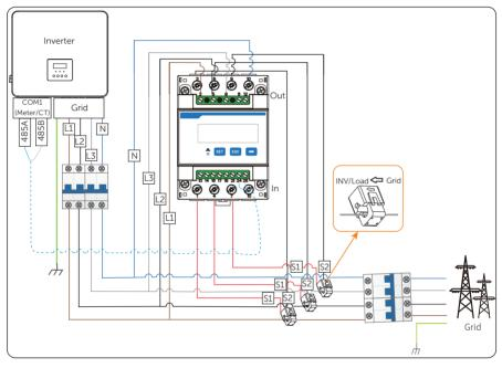
Figure 15-8 System wiring with CT-connected meter
