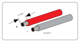
Figure 8-22 Stripping the PV cable
