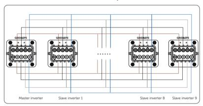
Figure 15-19 Power cable wiring with X3-PBOX-150kW-G2
