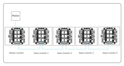
Figure 15-22 Communication wiring without X3-PBOX-150kW-G2
