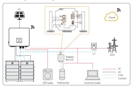
Figure 15-4 Adapter Box G2 wiring diagram
