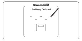
Figure 7-2 Marking the holes
