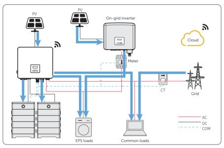
Figure 15-14 Power flowing when grid on and PV sufficient
