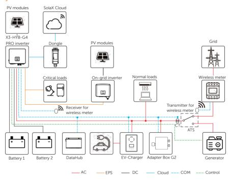
Figure 3-1 System diagram
