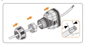
Figure 8-39 Threading the cable without the RJ45 terminal and striping
