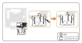
Figure 7-1 Installing the bracket
