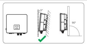
Figure 7-1 Correct installation
