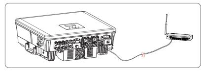
Figure 15-12 Connecting to DataHub
