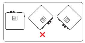
Figure 7-2 Incorrect installation
