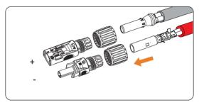
Figure 8-25 Threading the PV cable
