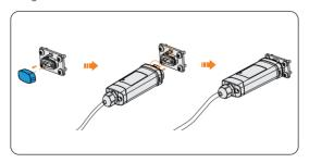
Figure 8-63 Connecting the dongle
