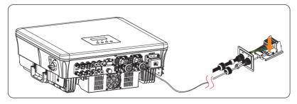
Figure 15-9 Connecting to EV-Charger
