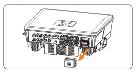
Figure 8-19 Removing the cap
