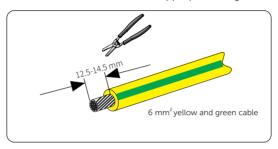
Figure 8-3 Striping the PE cable
