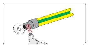
Figure 8-6 Shrinking the tubing
