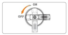
Figure 9-68 Turning off the DC switch
