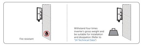
Figure 5-3 Installation carrier requirement
