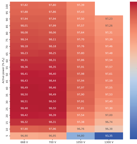
Fig. 8: Efficiency during charging (gridsave 92.0TL3-S)
