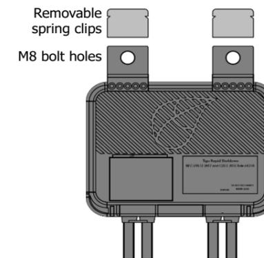
For frameless modules, use M8 bolts torqued to 10.2 Nm.
