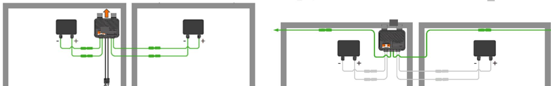
If connecting a TS4-A-2F to only one solar module, connect the TS4 #2 input cables to each other.
