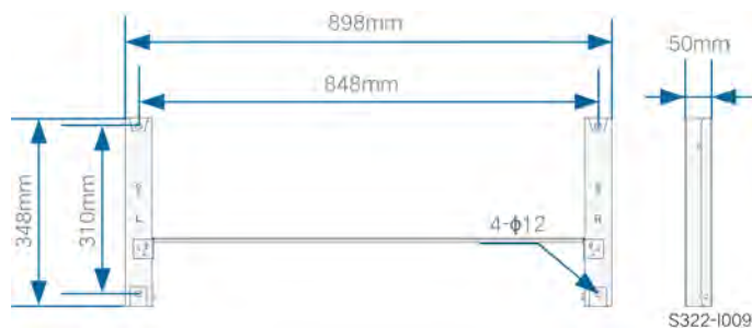
figure 4-1 Dimensions of Mounting-bracket
