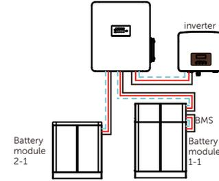
Connect with a MC0600 (BMS) and 4 HV10230 battery modules:
