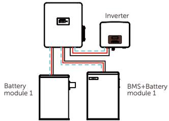
Connect with a T-BAT H 5.8 (BMS) and 3 HV11550 battery modules:
