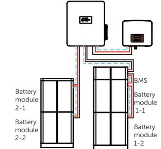
Connect with a MC0600 (BMS) and 6 HV10230 battery modules:
