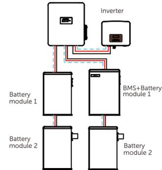
Connect with a T-BAT H 5.8 (BMS) and 5 HV11550 battery modules:
