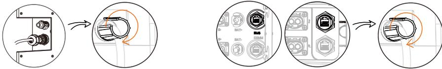
2) Connect the communication cable from the parallel box to the COMM/BMS/RS485 I communication port that is on the left side of the battery module.
