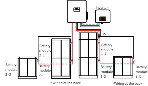
Connect with a MC0600 (BMS) and 8 HV10230 battery modules:
