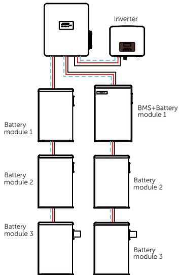
Connect with a T-BAT H 5.8 (BMS) and 7 HV11550 battery modules:
