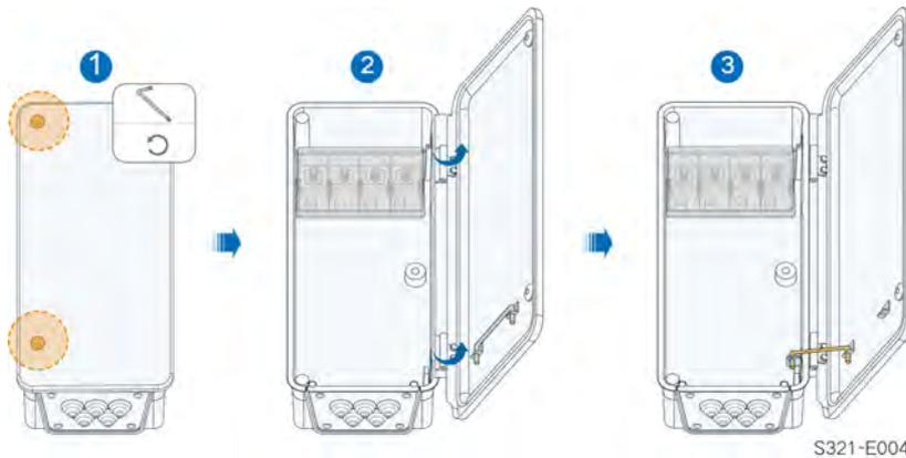
**i** The screws on the front cover are captive screws. When the front cover is opened, the screws remain on it.
