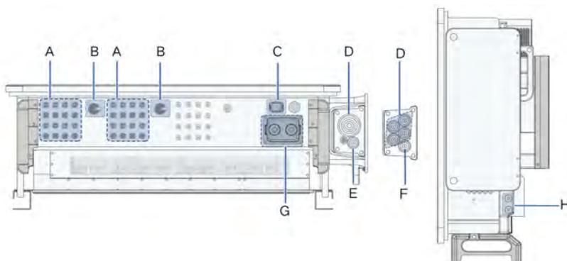
**figure 5-2** Terminal Description(SG75CX-P2)
