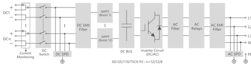
**figure 2-4** Circuit Diagram
