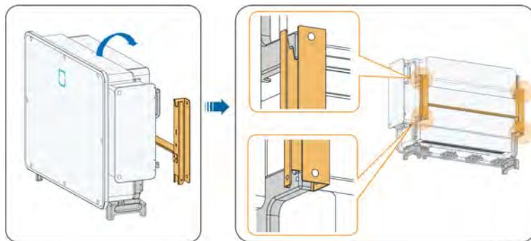
**step 3** Fix the inverter with screws.
