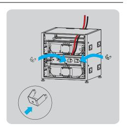
4. For the single stack installation systems, the power cables should be leaded to the "P+" and "P-"ports on A2 of the top and bottom LVL systems through the "Power" hole and also holes on the separation panels. All the other operations are as the same as the single system.
