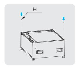
4. Pile A1 on A2. Make sure the holes at the bottom of A1 are just right above the alignment pins, and then lay A1 down on A2.
