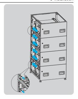
**Note:** LVL 2021 could be installed mixedly with LVL 15.4 in one stack (no matter which one is on the top) or both on the ground.
