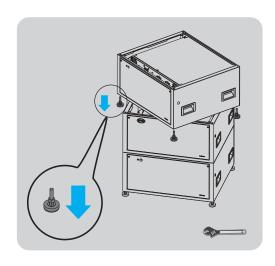
3. Insert two alignment pins on top of A1 (the bottom LVL) and A2 (the top LVL).
