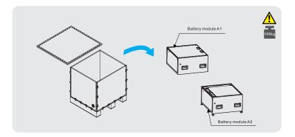
2. Remove the top panel of A1.
