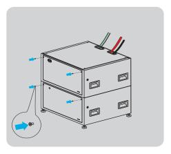
2. Insert the plastic bolts ( J in the delivery scope) on four corners of A2 top side. Meanwhile, fix the top panel of A2 with original screws there.
