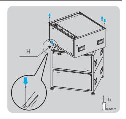
4. Lift A2 (the top LVL), and rotate it a little bit to make sure the holes of it right above the alignment pins of A1(the bottom LVL), and then put it down.
