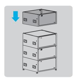
7. Connect the all the modules together with bonding strips. (three stripes each sides, and six strips in total. Torque, 4.5 Nm).
