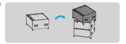
2. Remove four feet of A2 (the top LVL).
