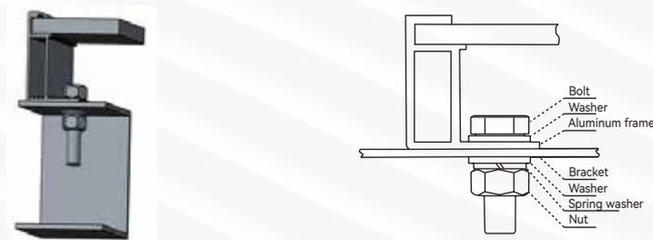
Figure 5 Bolt Installation of Mono-facial Modules
