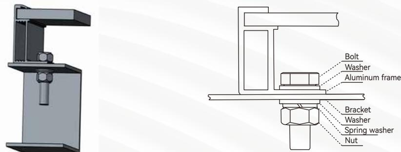
Figure 5 Bolt Installation of Mono-facial Modules
